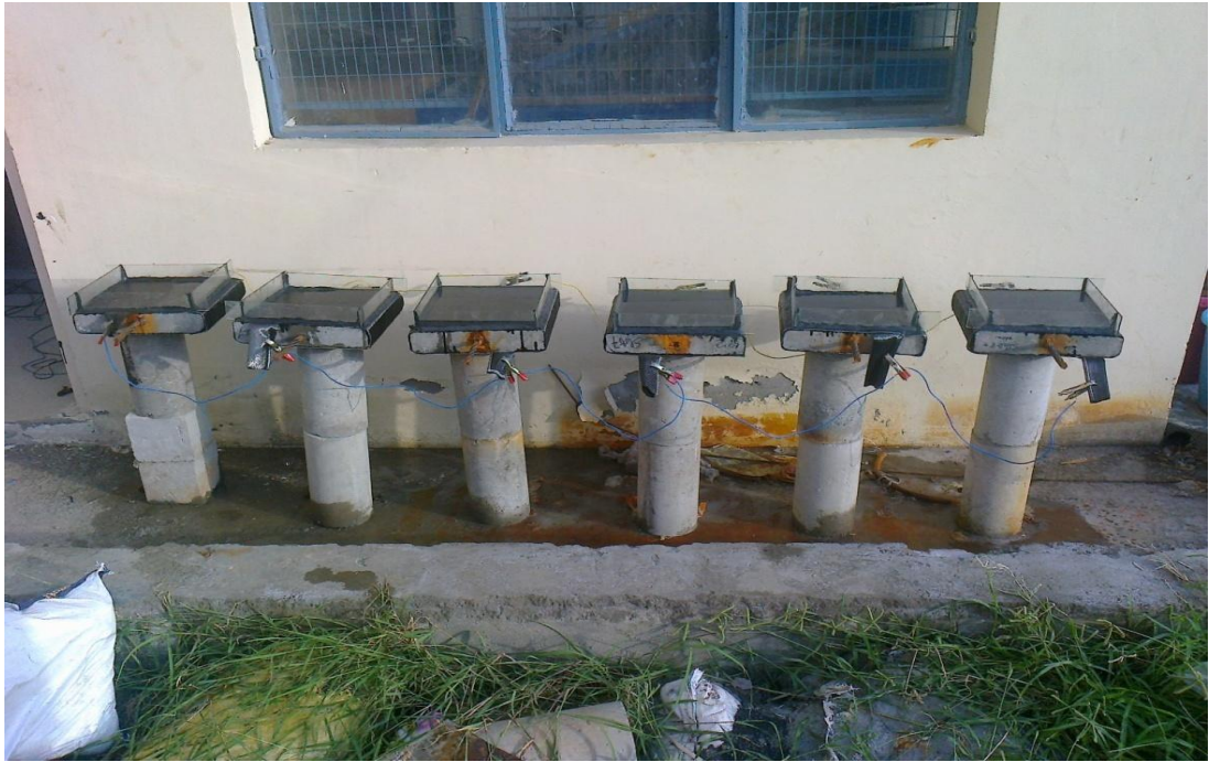
Fig.6.13 Set up of slab specimens for Active Protection
