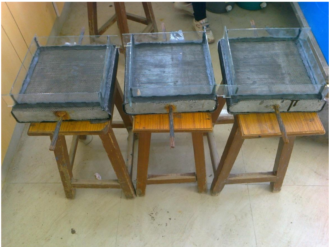
Fig. 6.14 Set up of Block Specimen for Passive Protection
