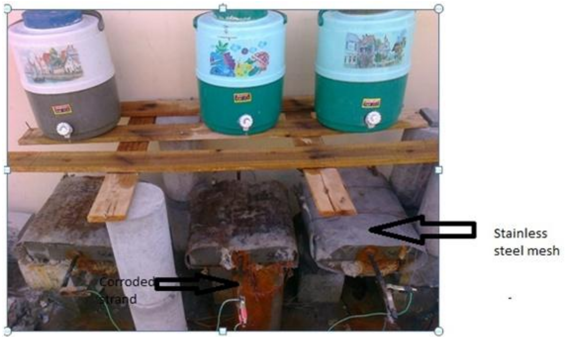
Fig. 6.3 Block Specimen subjected to 5% NaCl Solution
