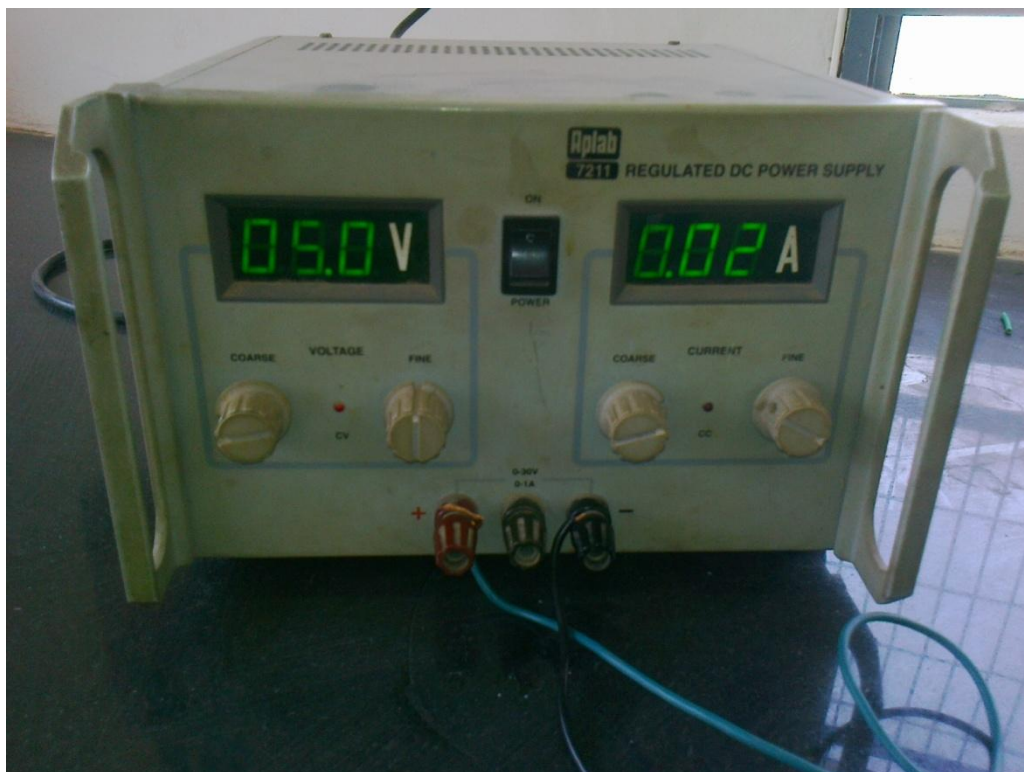
Fig. 6.4 Power supply used to accelerate Corrosion in specimens
