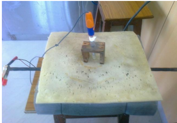
Fig.6.6 Half cell measurement on block specimen
