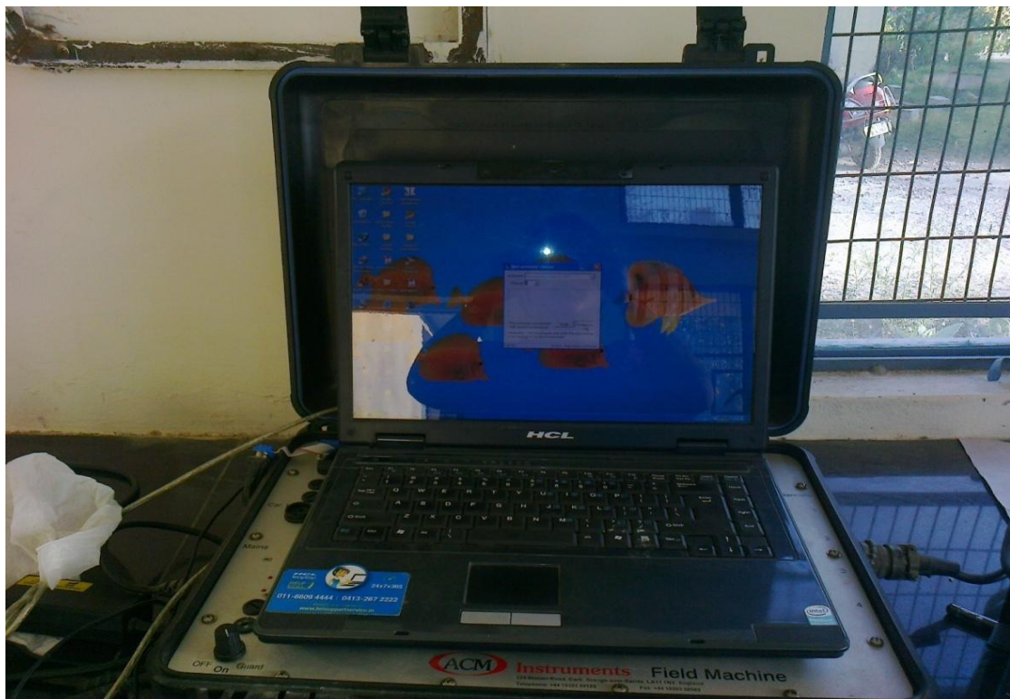
Fig.6.5 ACM Corrosion Analyser Field Machine
