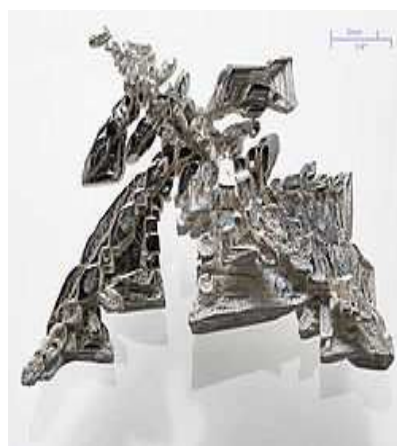
Figure 1.1 Electrolytically refined silver
