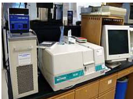
Figure 2.4 DU640 UV/Vis spectrophotometer.
