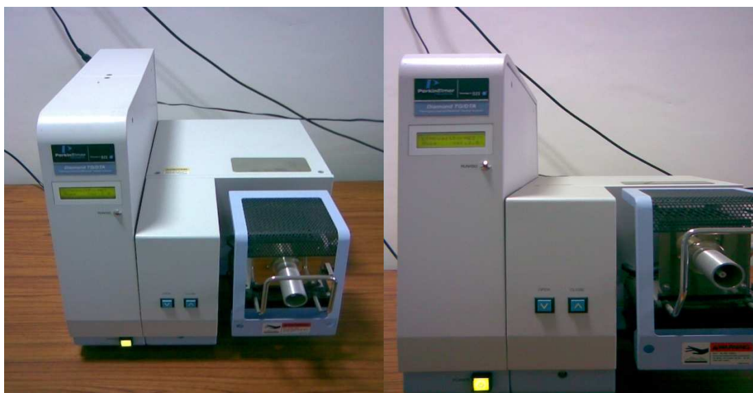
Figure 2.6 Diamond Pyris TGA/DTA thermal analyzer
