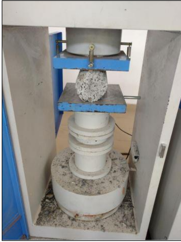
Figure 3.5. Experimental set up for split tensile strength test
