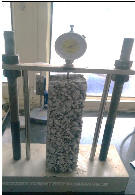
Figure 3.9. Experimental set up of measuring length gauge
