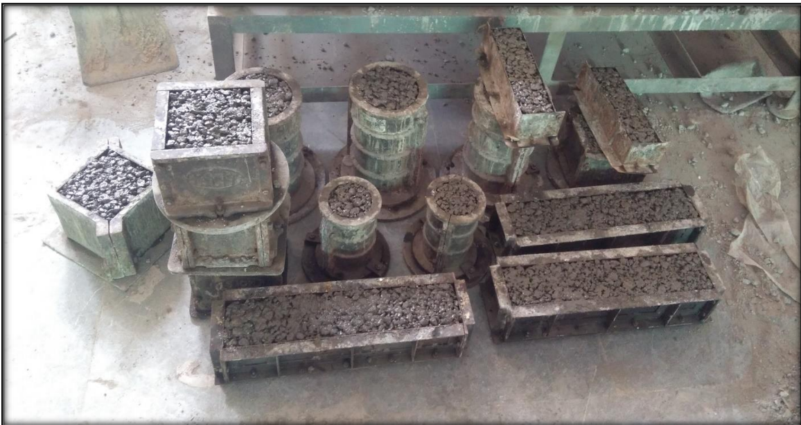
Figure 3.3. Casting of NFC specimens
