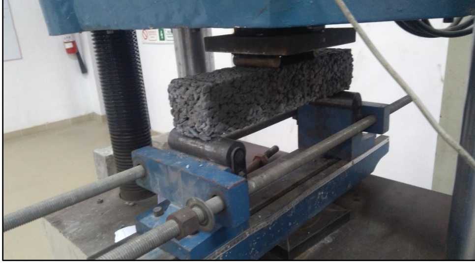
Figure 3.6. Experimental set up for the flexural strength test
