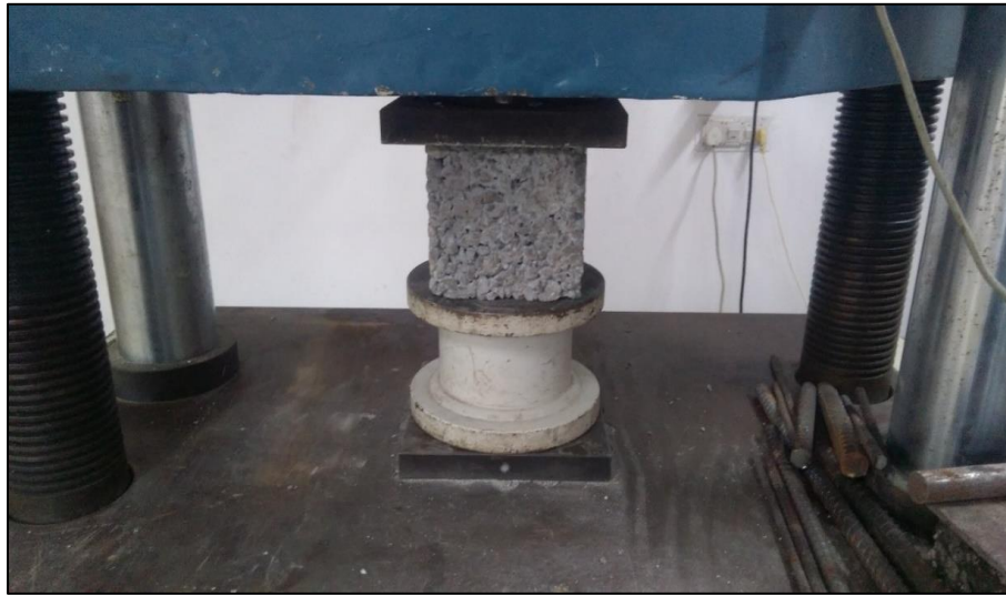
Figure 3.4. Strength test of NFC Sample in progress in the UTM
