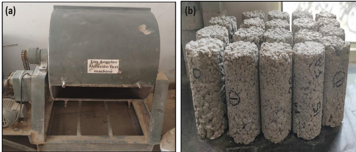
Figure 3.10. (a) Experimental set up of abrasion resistance (b) NFC specimens prepared for abrasion testing
