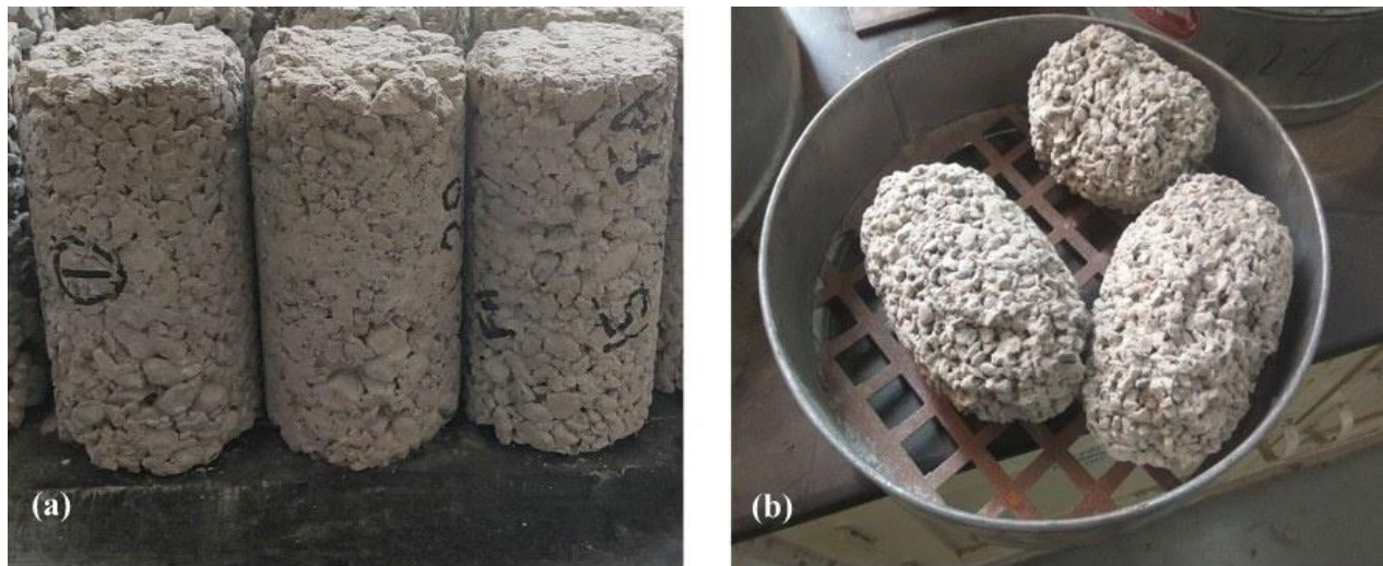
Figure 4.16. (a) NFC specimens before abrasion test and (b) NFC specimens after abrasion test
