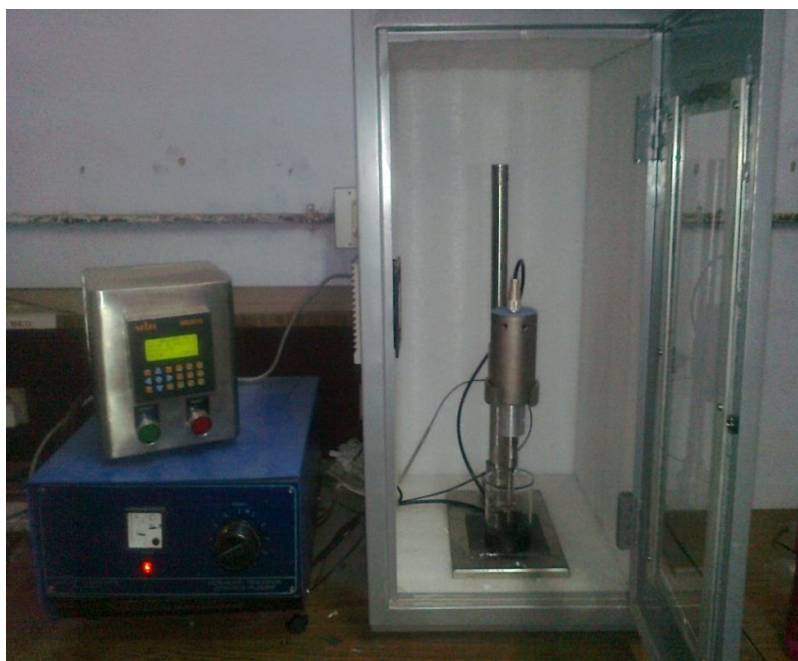
Figure A2: Ultrasonicator for the sonication of nanofluid for required time.
