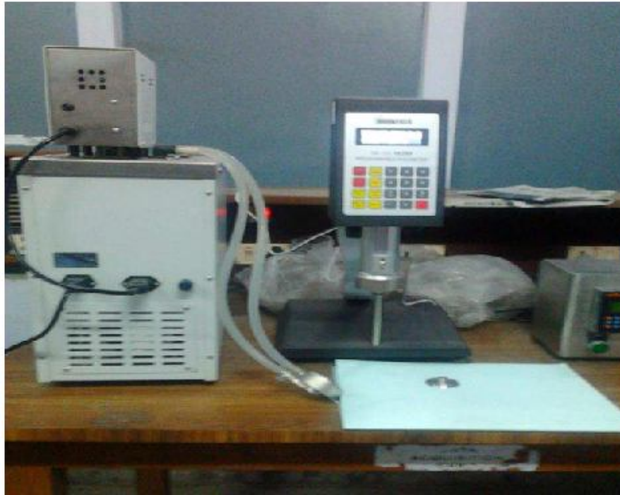
Figure A3: Brookfield DV III Rheometer with circulating bath.
