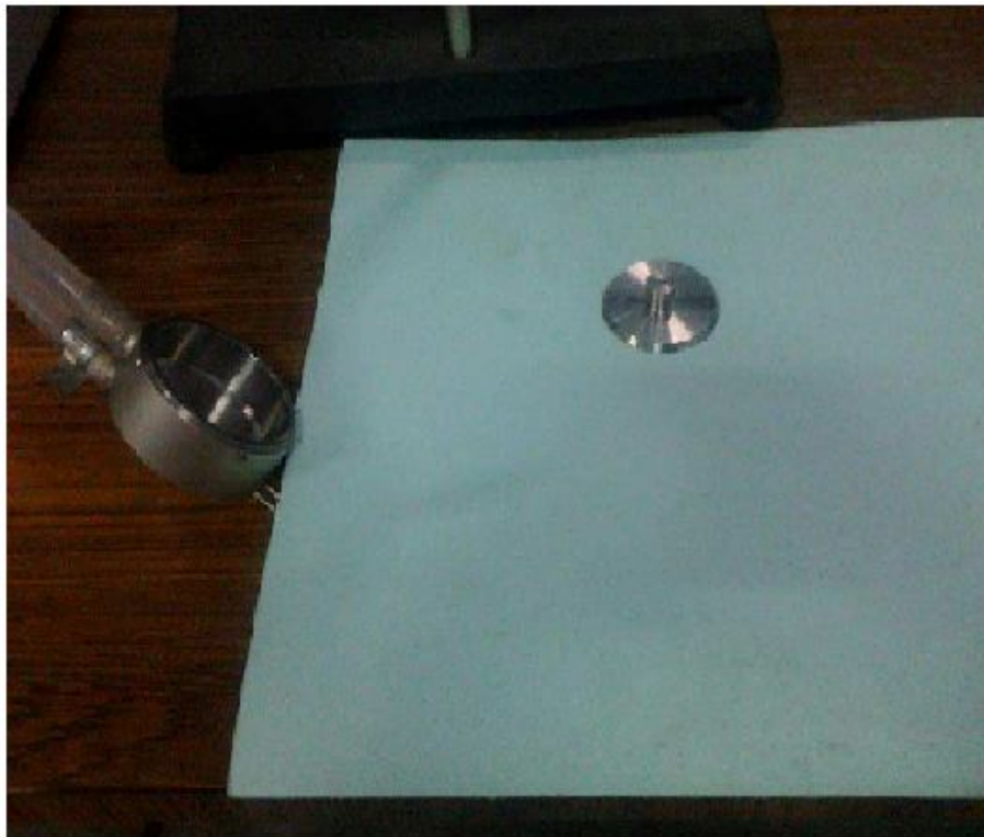
Figure A4: Cup and Cone arrangement of Rheometer.
