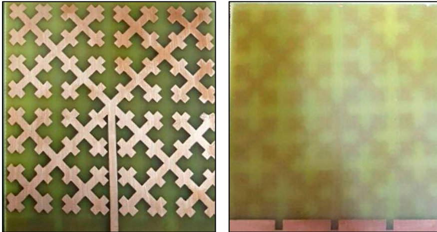
Figure5.2 Photograph of front and back view of the fabricated antenna with reduced size
