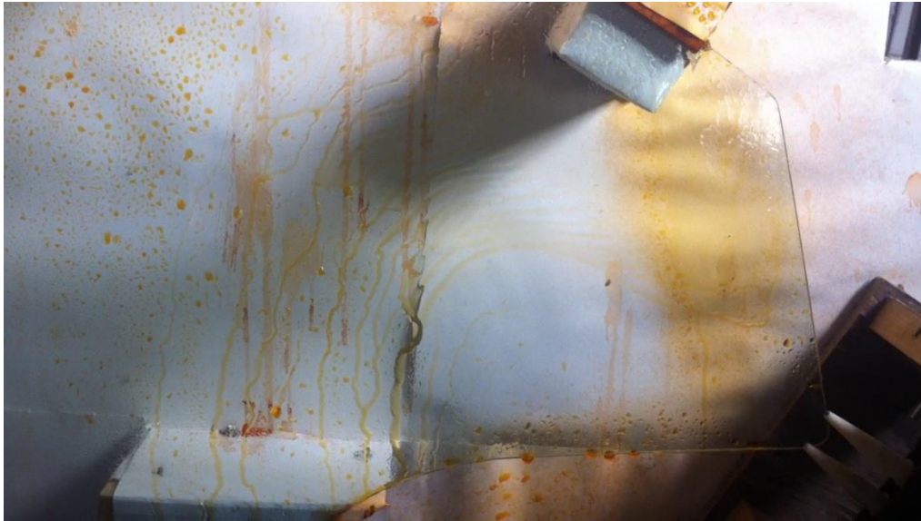
Fig. 4.19 : Area Cleaned 100 mm 2 at outlet air velocity = 30 m/s with Inlet Diameter=1 mm, Outlet Diameter=9 mm, Throat Length=30 mm, Converging Length=40 mm & Impinging Angle=0 0
