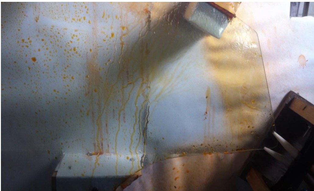
Fig. 4.20 : Area Cleaned 158 mm 2 at outlet air velocity = 35 m/s with Inlet Diameter=1 mm, Outlet Diameter=9 mm, Throat Length=30 mm, Converging Length=40 mm & Impinging Angle=0 0
