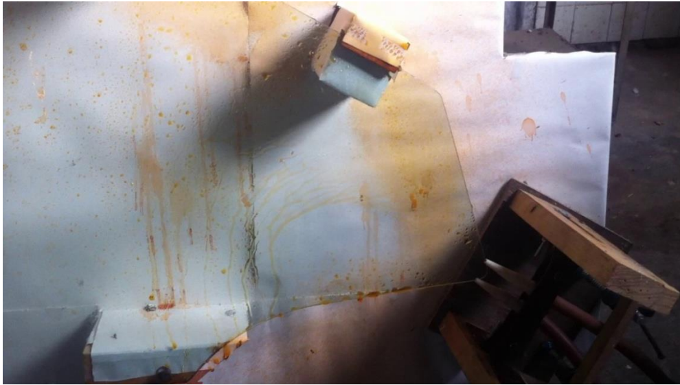
Fig. 4.16 : Area Cleaned 218 mm 2 at outlet air velocity = 30 m/s with Inlet Diameter=1 mm, Outlet Diameter=9 mm, Throat Length=30 mm, Converging Length=40 mm & Impinging Angle=0 0
