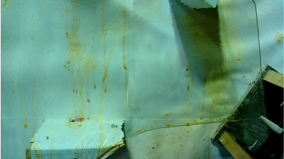
Fig. 4.15 : Area Cleaned 272 mm 2 at outlet air velocity = 40 m/s with Inlet Diameter=1 mm, Outlet Diameter=9 mm, Throat Length=30 mm, Converging Length=40 mm & Impinging Angle= 0^\circ
