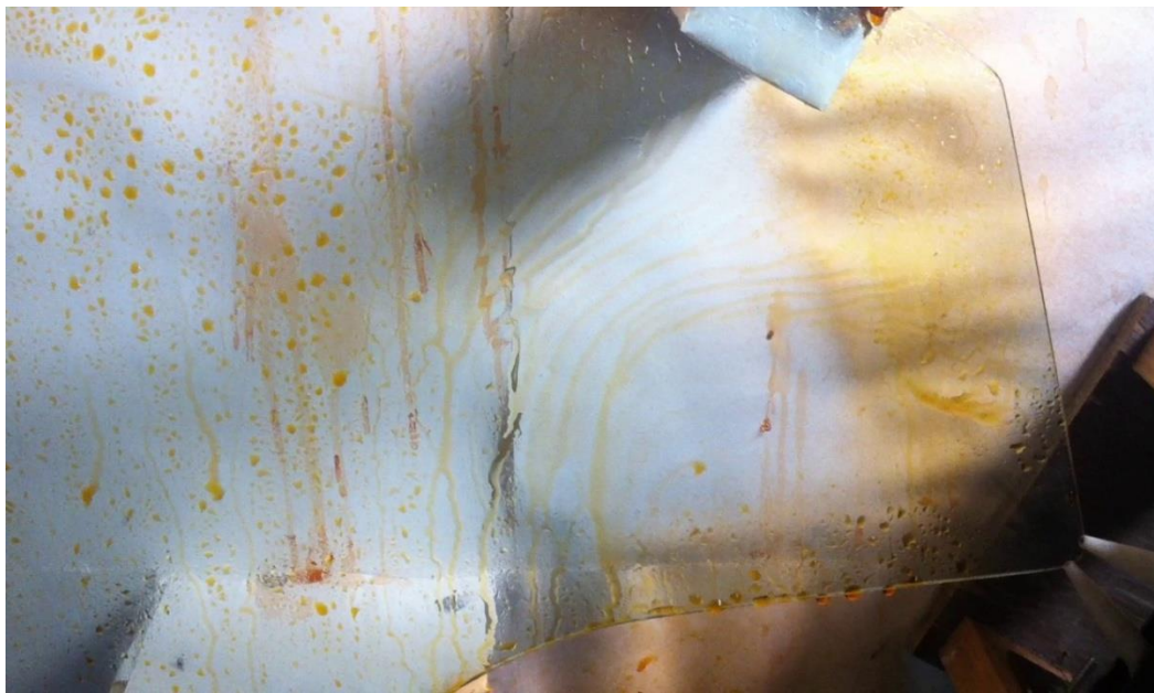
Fig. 4.23 : Area Cleaned 186 mm 2 at outlet air velocity = 35 m/s with Inlet Diameter=1 mm, Outlet Diameter=9 mm, Throat Length=30 mm, Converging Length=40 mm & Impinging Angle=0 0
