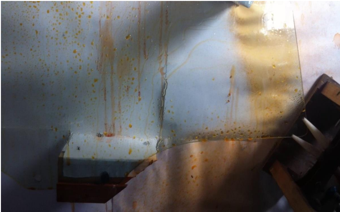
Fig. 4.21 : Area Cleaned 204 mm 2 at outlet air velocity = 40 m/s with Inlet Diameter=1 mm, Outlet Diameter=9 mm, Throat Length=30 mm, Converging Length=40 mm & Impinging Angle=0 0
