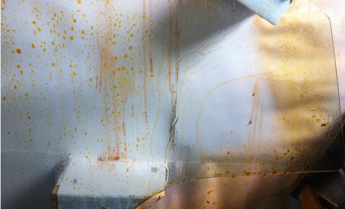
Fig. 4.24 : Area Cleaned 234 mm 2 at outlet air velocity = 40 m/s with Inlet Diameter=1 mm, Outlet Diameter=9 mm, Throat Length=30 mm, Converging Length=40 mm & Impinging Angle=0 0
