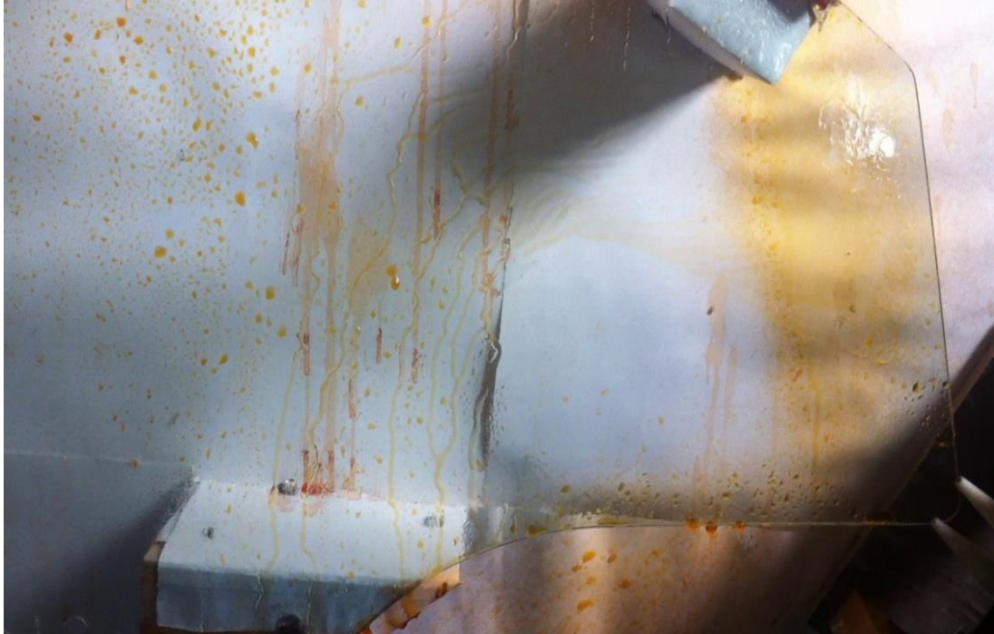
Fig. 4.18 : Area Cleaned 370 mm 2 at outlet air velocity = 40 m/s with Inlet Diameter=1 mm, Outlet Diameter=9 mm, Throat Length=30 mm, Converging Length=40 mm & Impinging Angle=0 0
