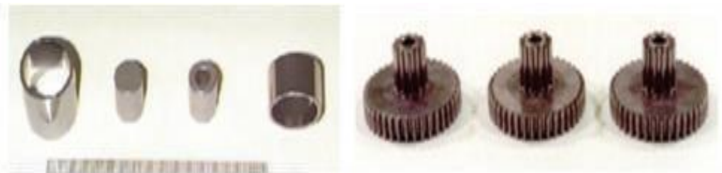
Figure 1.5: Various steel parts sintered by microwave processing.
