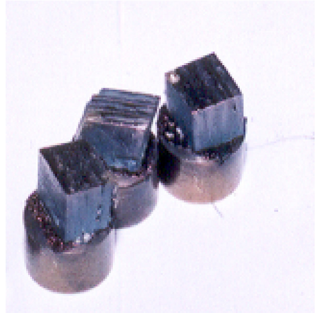
Fig. 1. Specimen preparation: 4 layers of sheets bonded for gold coating.
