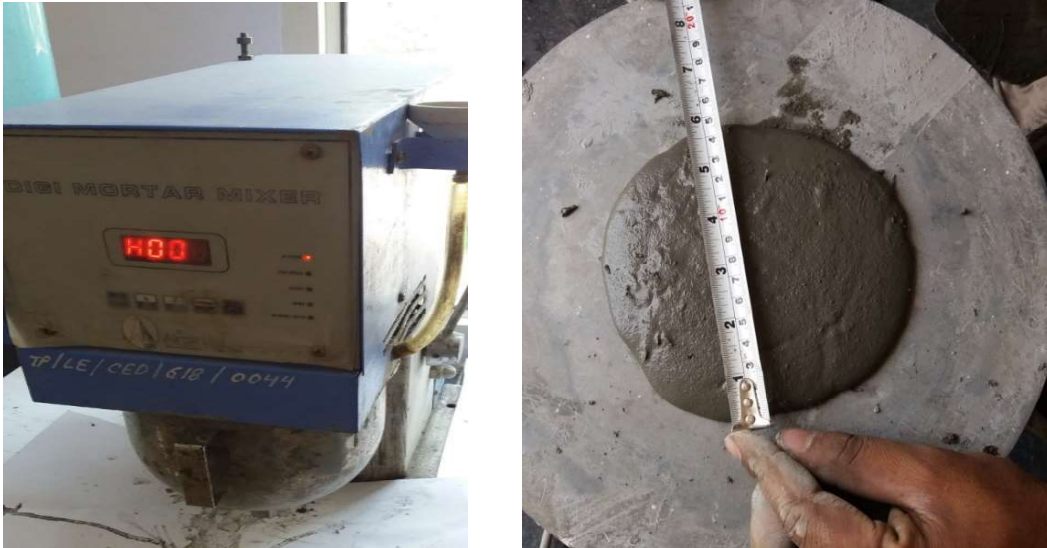
Figure 3.7 (a): Preparation of HPFRCC in digi mortar mixer. Figure 3.7 (b): Measurement of flowability.
