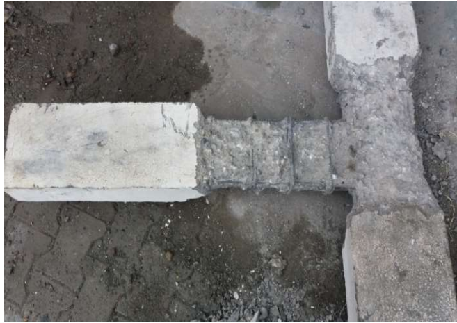
Figure 3.12 (b): Specimen ready for retrofitting.
