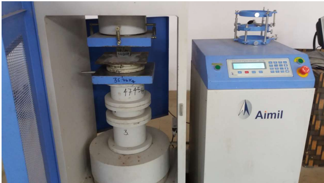
Figure 3.7( d): Testing of cube.
