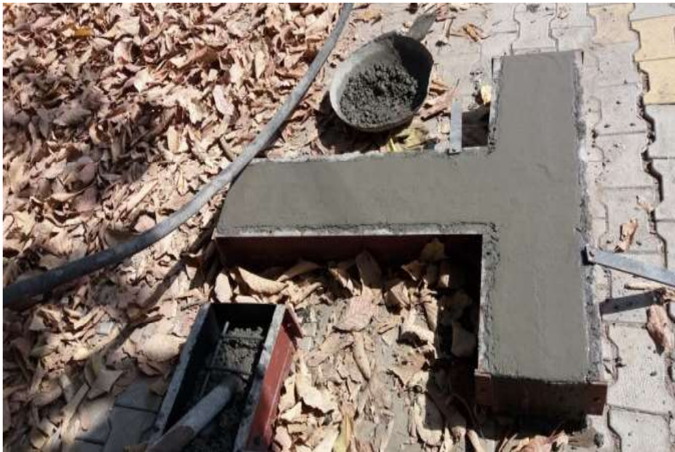
Figure 3.9 (c): Casting of specimen.
