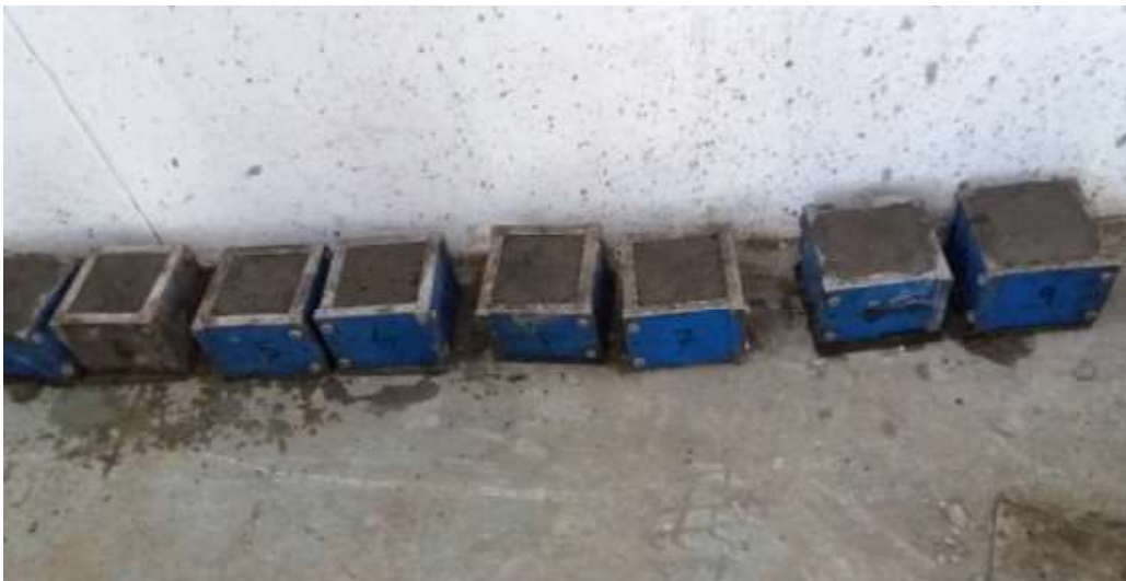
Figure 3.7 (c): Casting of cubes.
