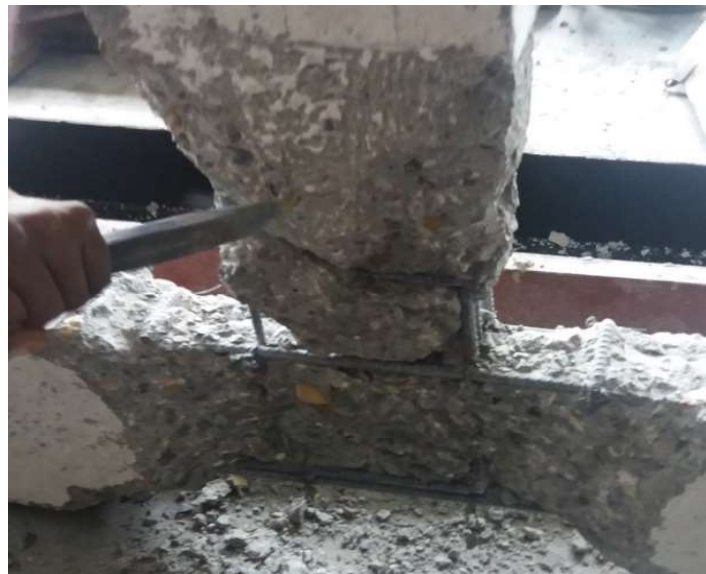
Figure 3.12 (a): Chipping off cover of specimen in central region.
