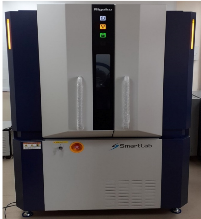
Fig. 3.2: Smart lab SE (Rigaku) setup for XRD.
