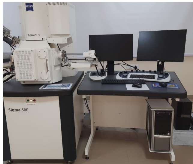
Fig. 3.3: Carl Zeiss Sigma 500 FEG-SEM setup for microstructure observation.
