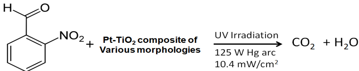
Scheme 1. Diagrammatic representation for the photodegradation of nitrobenzaldehyde using various Pt-TiO 2 composites under UV light irradiation.
