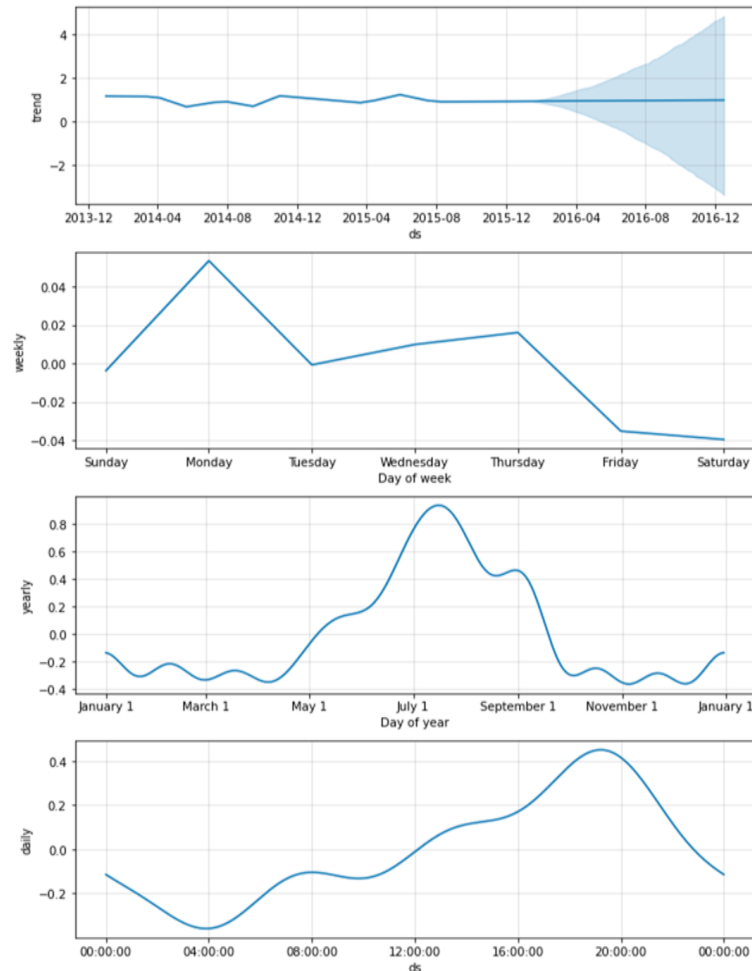
Figure 5.13: Charts (top to bottom): Trend, Weekly, Yearly and Daily-datasets used in the Prophet model
