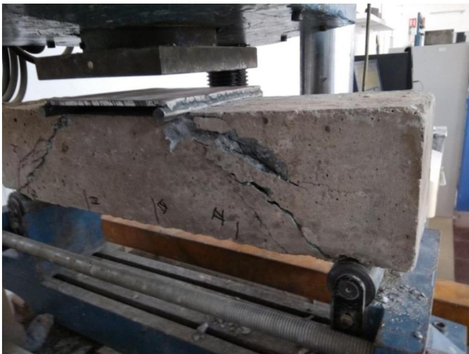
Figure 4.18 Cracks in S3 (2) of grade M35 beam at ultimate load 84.15kN
