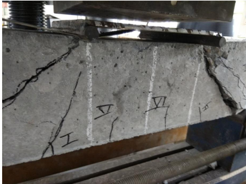
Figure 4.19 Cracks in S4 (1) of grade M30 beam at ultimate load 82.88kN
