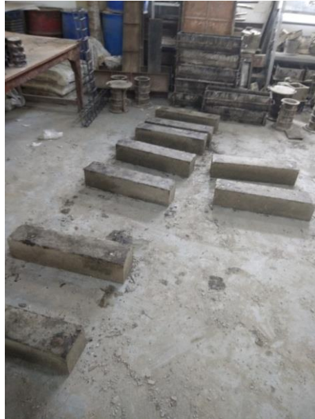
Figure 3.11 Beam specimens after dismantling
