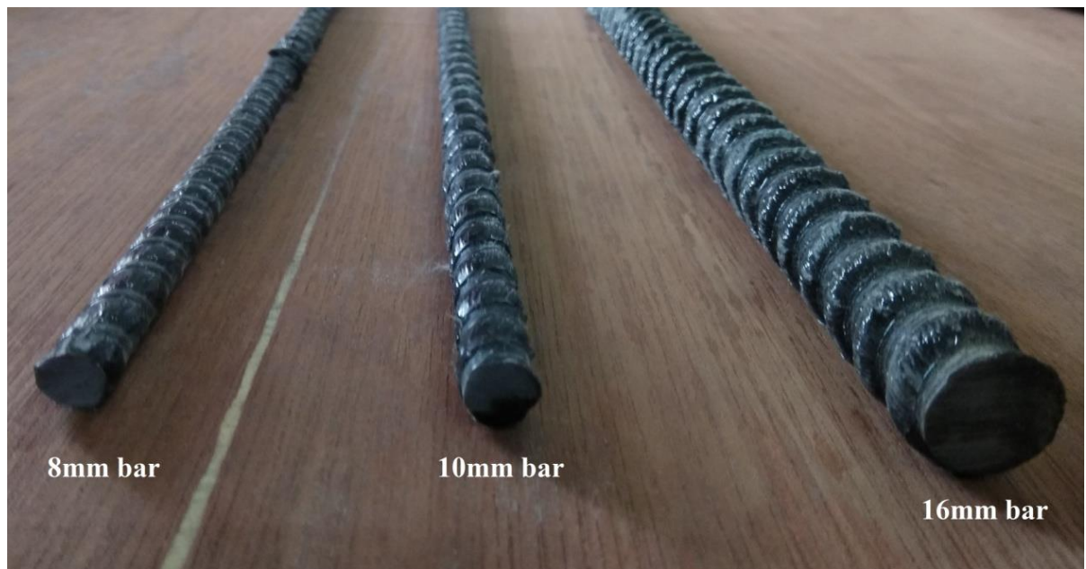
Figure 3.2 GFRP bars of different diameters
