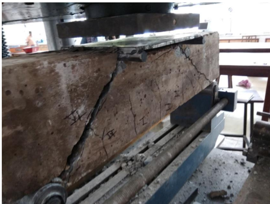
Figure 4.32 Cracks in G3 (2) of grade M30 beam at ultimate load 66.17kN
