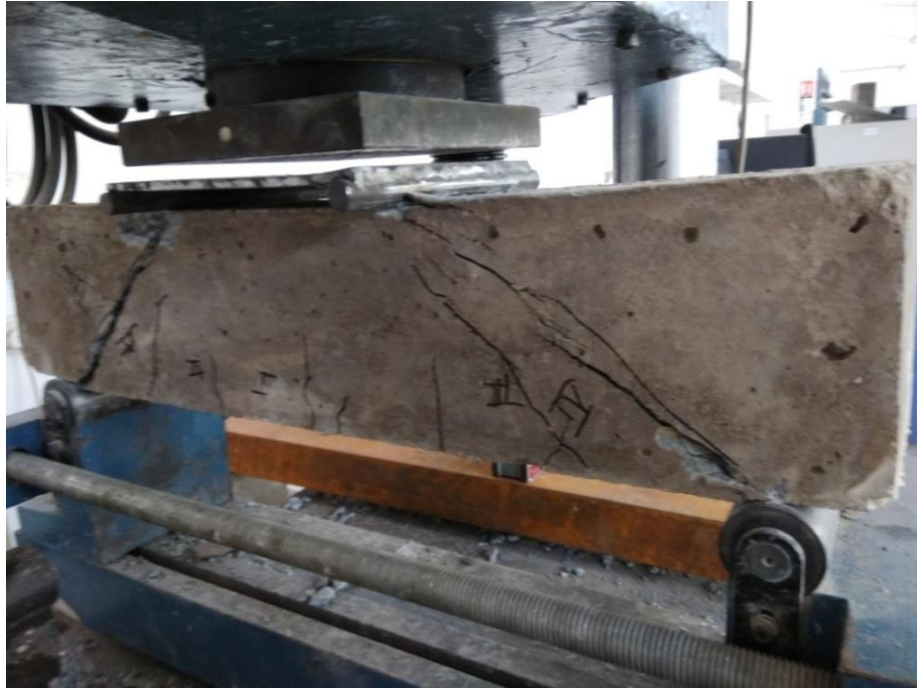
Figure 4.17 Cracks in S3 (1) of grade M35 beam at ultimate load 95.92kN
