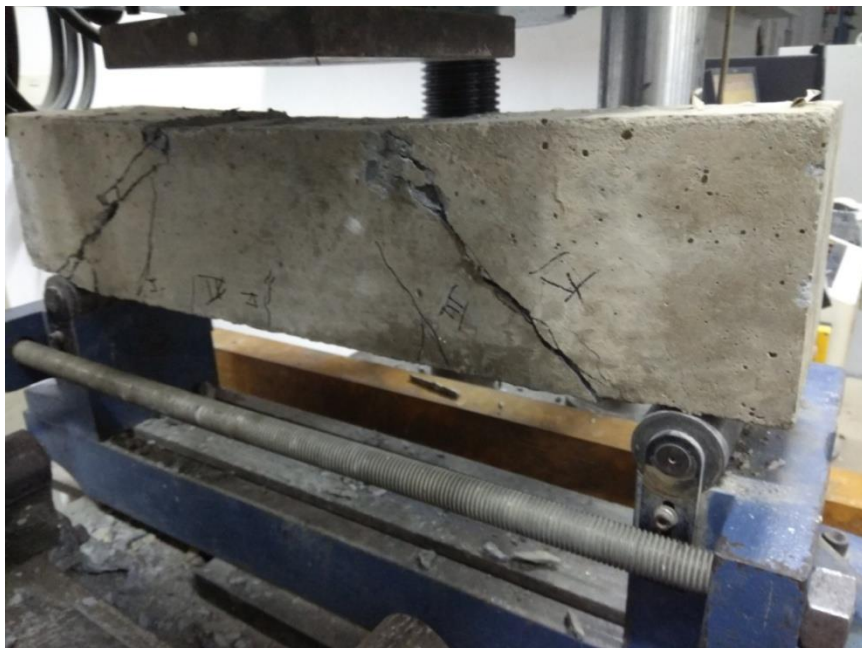
Figure 4.16 Cracks in S3 (2) of grade M30 beam at ultimate load 80.8kN
