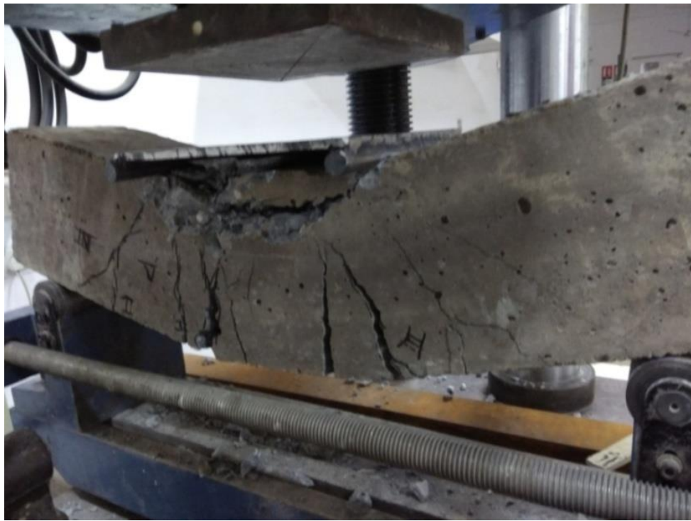
Figure 4.9 Cracks in S1 (1) of grade M35 beam at ultimate load 50.24kN
