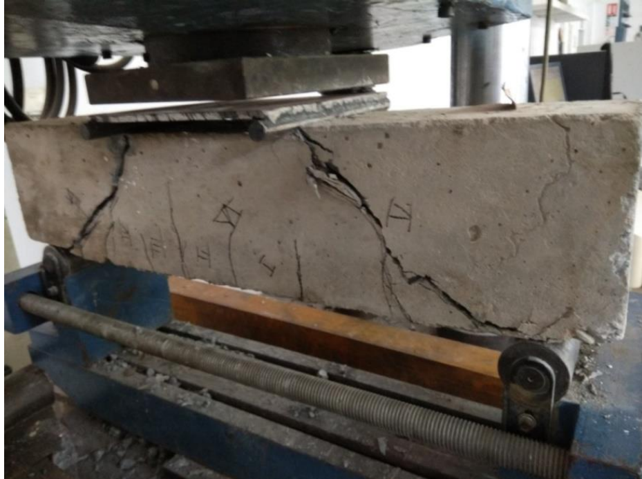
Figure 4.31 Cracks in G3 (1) of grade M30 beam at ultimate load 68.23kN
