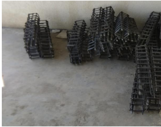
Figure 3.9 Steel and GFRP arrangements of beams
