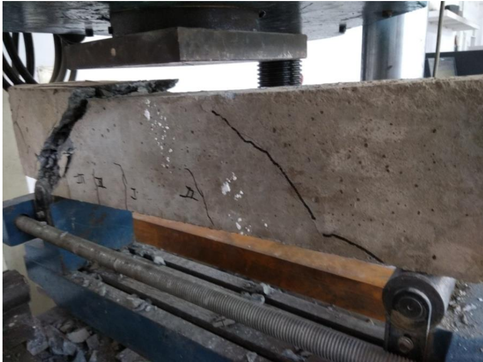
Figure 4.35 Cracks in G4 (1) of grade M30 beam at ultimate load 55.77kN
