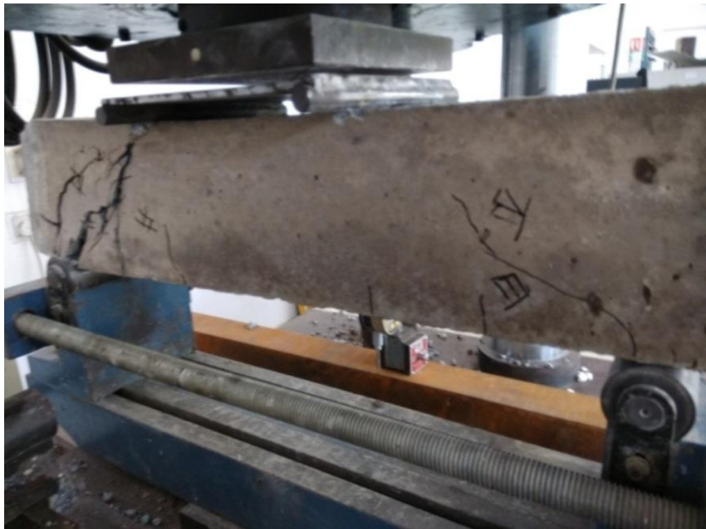
Figure 4.21 Cracks in S4 (1) of grade M35 beam at ultimate load 89.00kN
