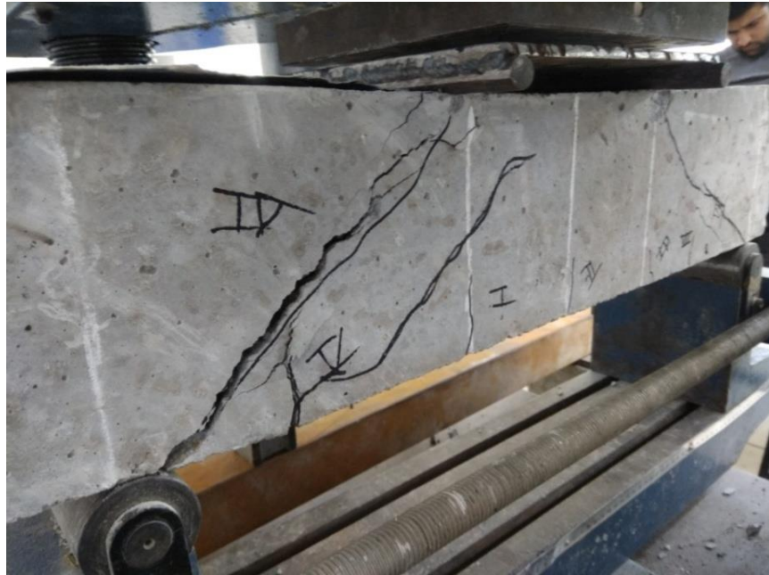
Figure 4.15 Cracks in S3 (1) of grade M30 beam at ultimate load 79.14kN
