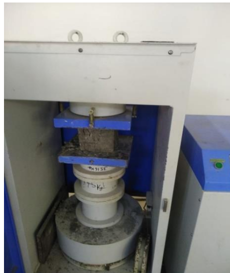
Figure-3.4 Strength testing of a cube in CTM (compressive)
