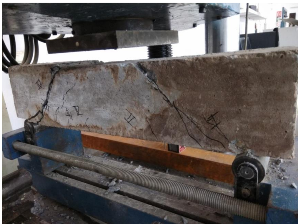
Figure 4.22 Cracks in S4 (2) of grade M35 beam at ultimate load 98.63kN
