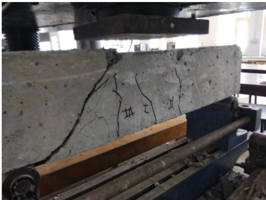
Figure 4.26 Cracks in G1 (2) of grade M35 beam at ultimate load 52.57kN
