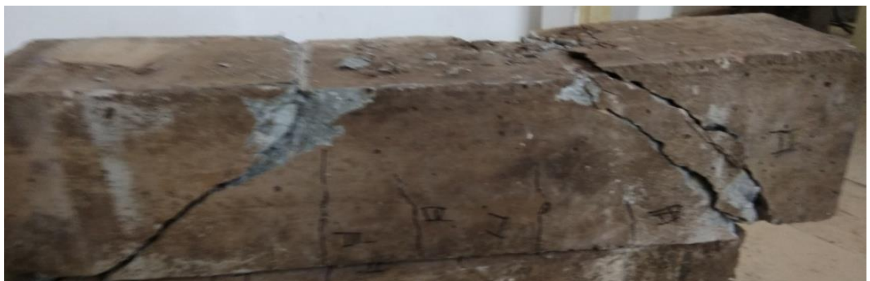
Figure 4.28 Cracks in G2 (2) of grade M30 beam at ultimate load 63.18kN
