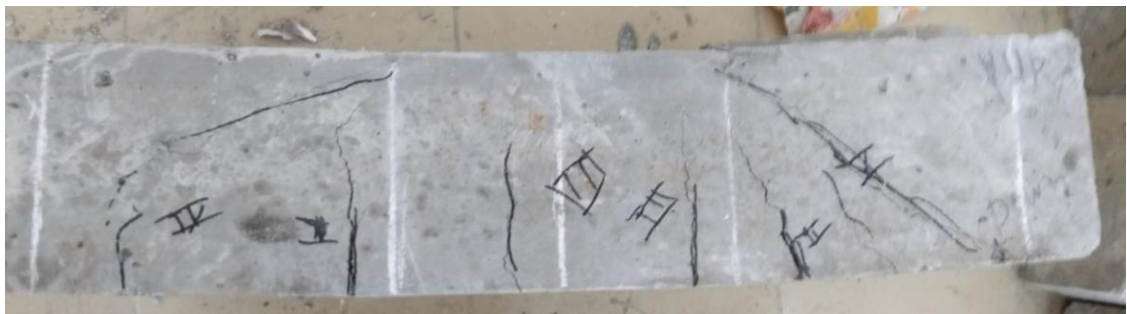
Figure 4.7 Cracks in S1 (1) of grade M30 beam at ultimate load 46.95kN
