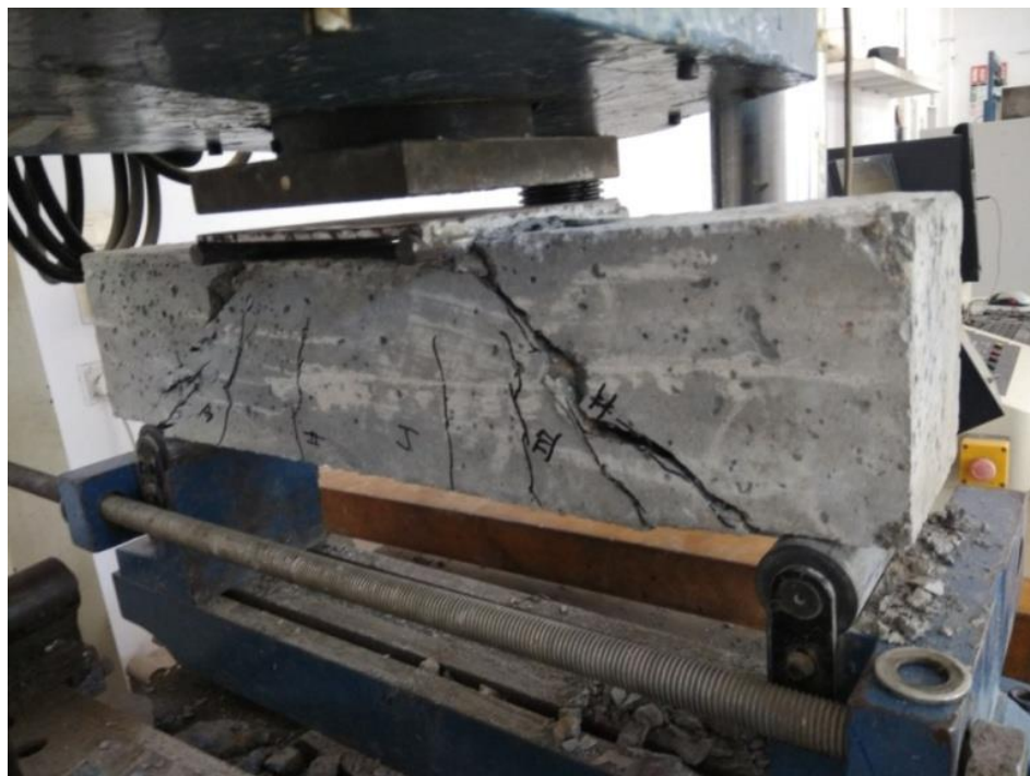
Figure 4.30 Cracks in G2 (2) of grade M35 beam at ultimate load 66.26kN
