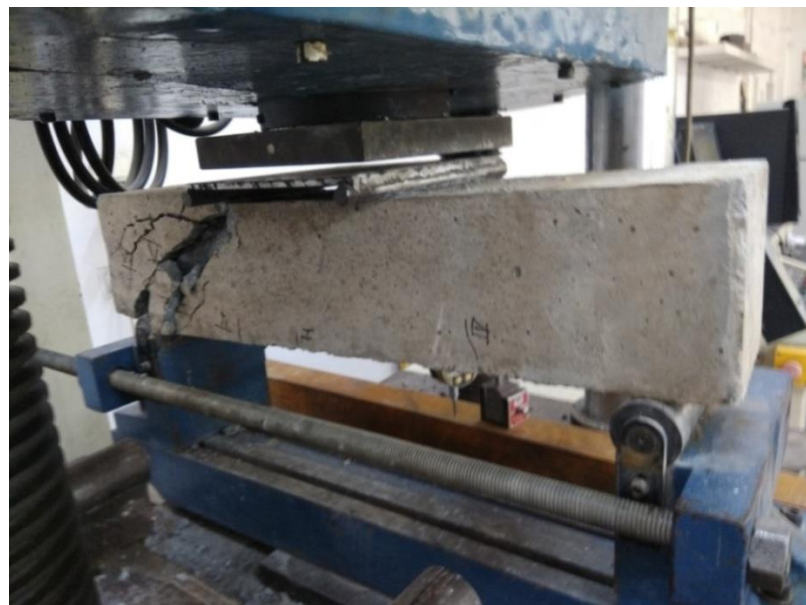
Figure 4.20 Cracks in S4 (2) of grade M30 beam at ultimate load 85.11kN
