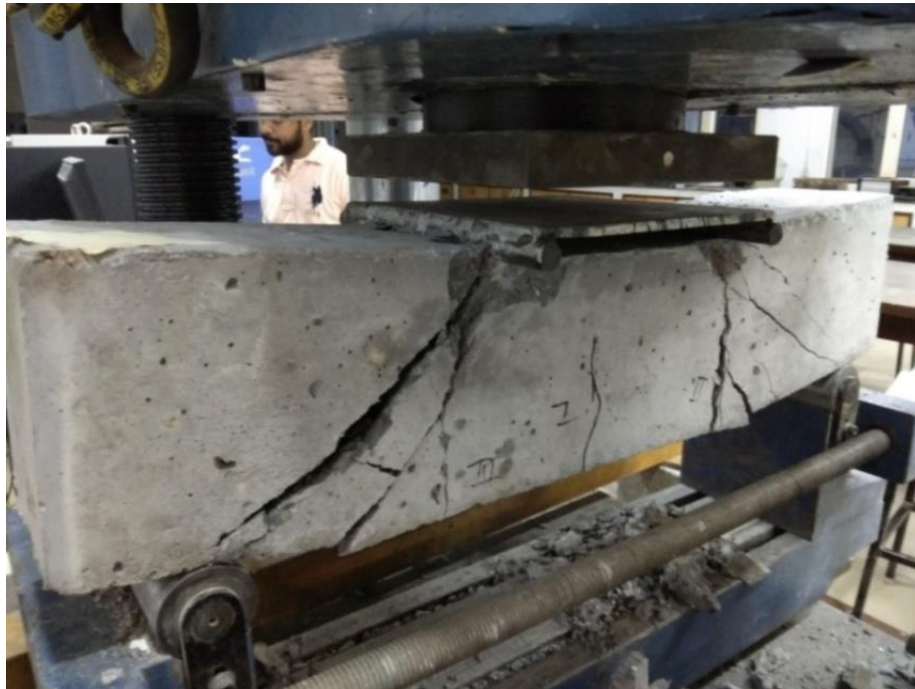
Figure 4.25 Cracks in G1 (1) of grade M35 beam at ultimate load 53.67kN
