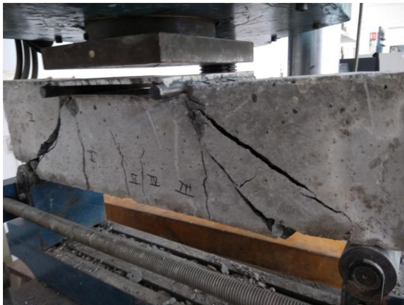
Figure 4.23 Cracks in G1 (1) of grade M30 beam at ultimate load 56.75kN
