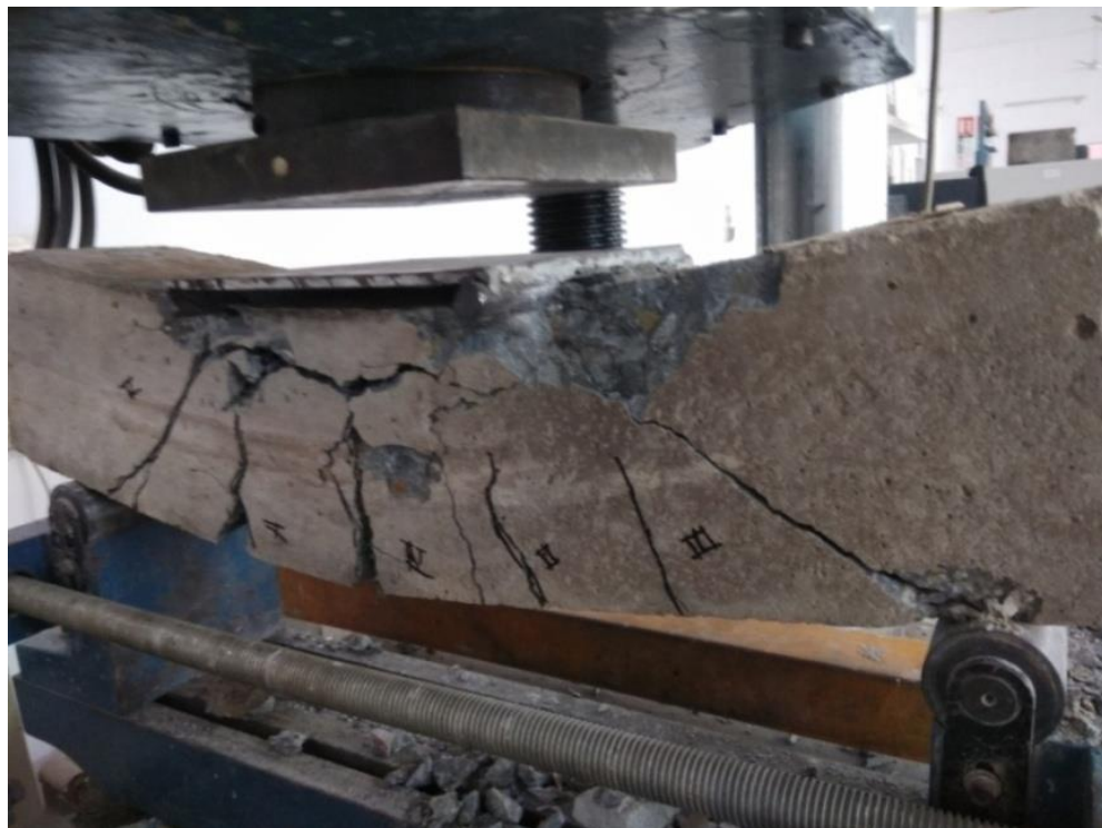
Figure 4.10 Cracks in S1 (2) of grade M35 beam at ultimate load 52.16kN
