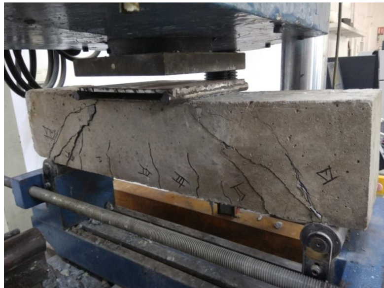
Figure 4.12 Cracks in S2 (2) of grade M30 beam at ultimate load 72.84kN
