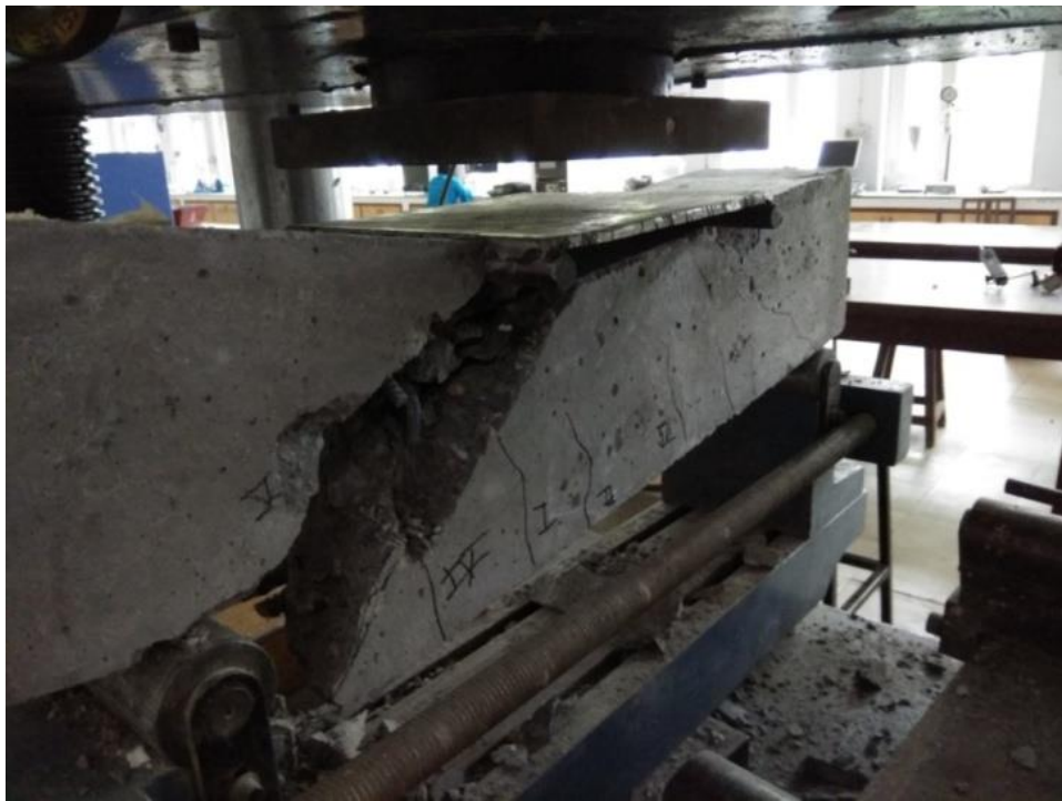
Figure 4.29 Cracks in G2 (1) of grade M35 beam at ultimate load 49.92kN
