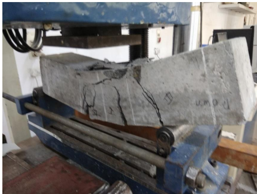
Figure 4.8 Cracks in S1 (1) of grade M30 beam at ultimate load 48.21kN
