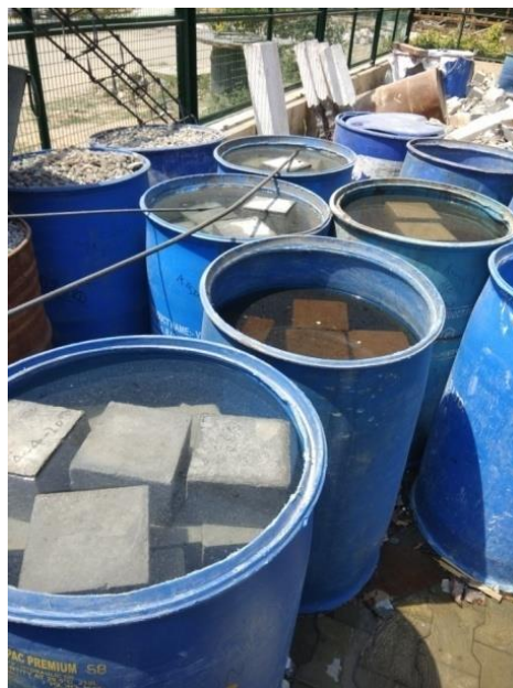
Figure 3.12 Prepared beams were placed in plastic tanks for 28 days curing.
