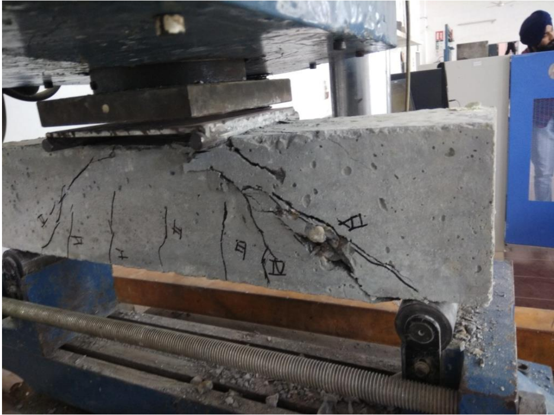
Figure 4.33 Cracks in G3 (1) of grade M35 beam at ultimate load 89.91kN
