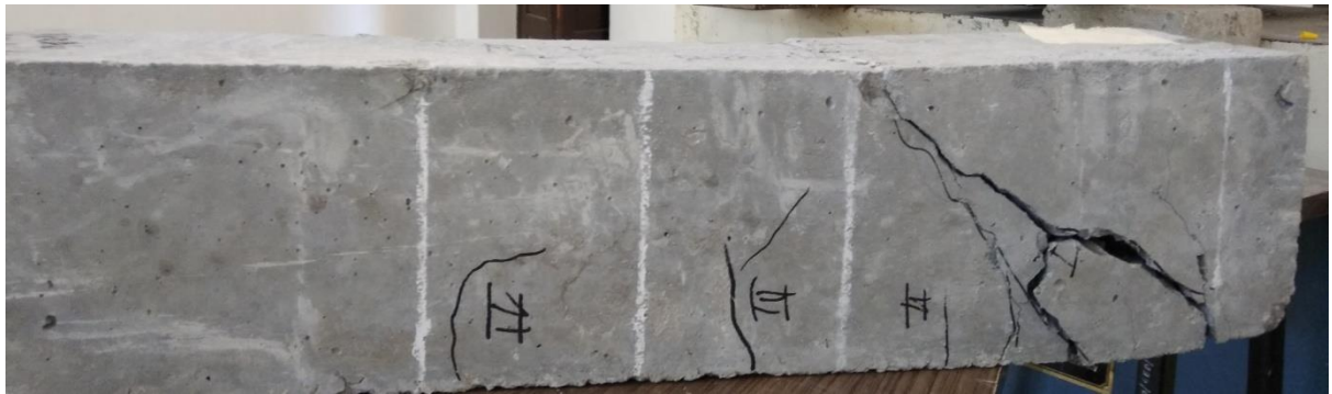
Figure 4.11 Cracks in S2 (1) of grade M30 beam at ultimate load 54.85kN
