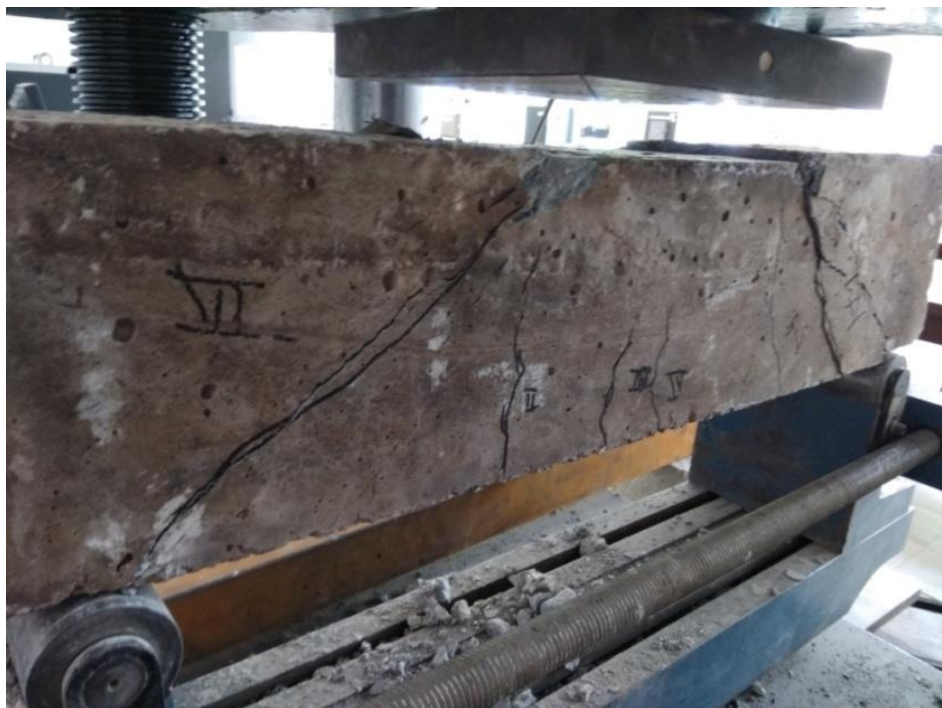
Figure 4.27 Cracks in G2 (1) of grade M30 beam at ultimate load 67.75kN
