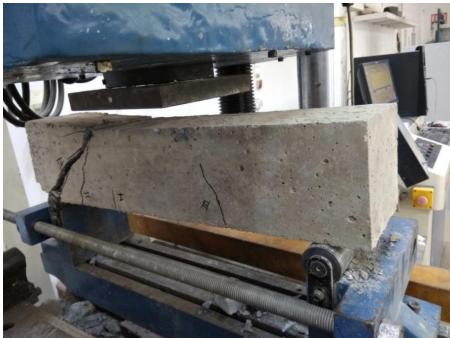
Figure 4.14 Cracks in S2 (2) of grade M35 beam at ultimate load 58.03kN
