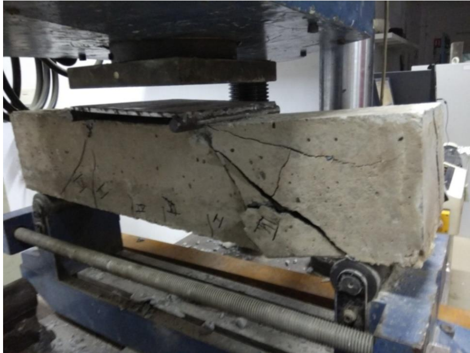
Figure 4.13 Cracks in S2 (1) of grade M35 beam at ultimate load 78.61kN
