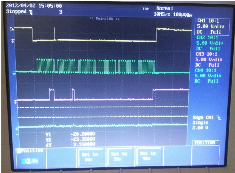
Figure 44: SPI Interface Waveform
