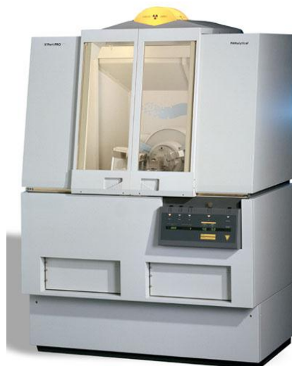
Figure 3.1: X-Ray Diffractometer by PANalytical X'Pert PRO with \text{CuK}\alpha ( \lambda = 1.5418 \text{ \AA} ) radiation.
