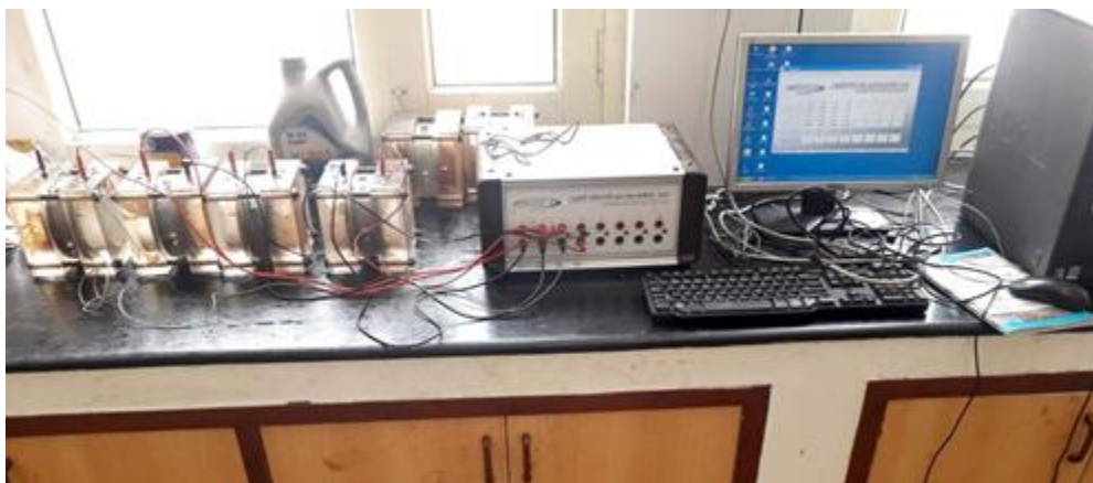
Figure 3.9. Setup for Rapid Chloride Permeability Test.
