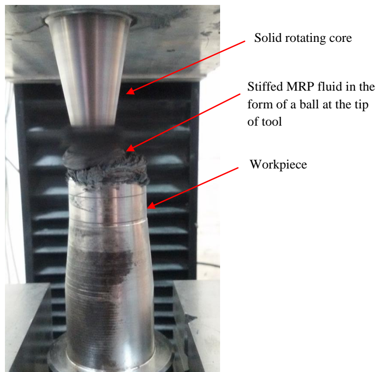
Figure 4.3: Ball end solid rotating core tool while performing the finishing operation
