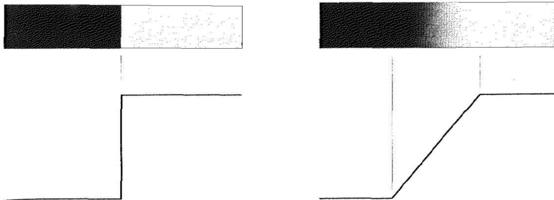
Figure-6.1: Edge profile of a gray scale image. [5]
