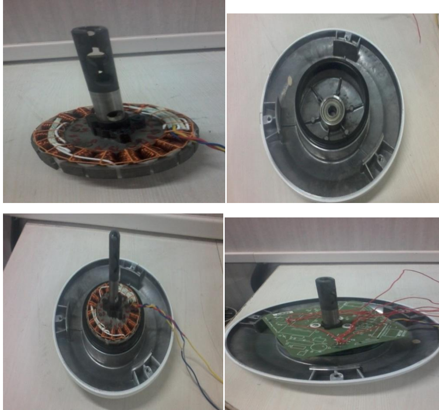
Fig. 4.6 A photo of assembling of ceiling fan
