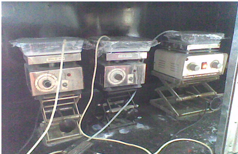
F 5.4 Experimental UV chamber with glass reactors
