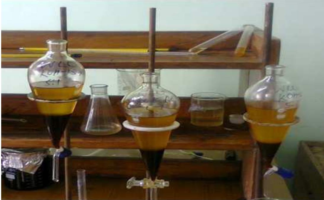
Fig 4.1: Separation of methyl ester at different KOH concentration
