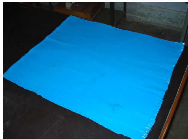
Fig. 4.15 The fully cured sheet with epoxy coating
