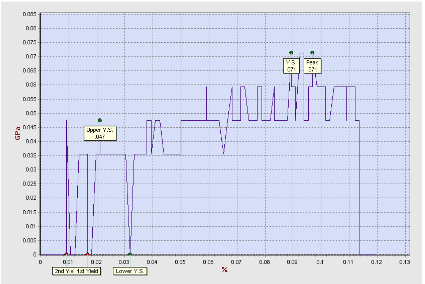
Fig.6.102 Stress vs Strain graph of sample loaded at 40% of U.T.L (NaOH Tank T2)
