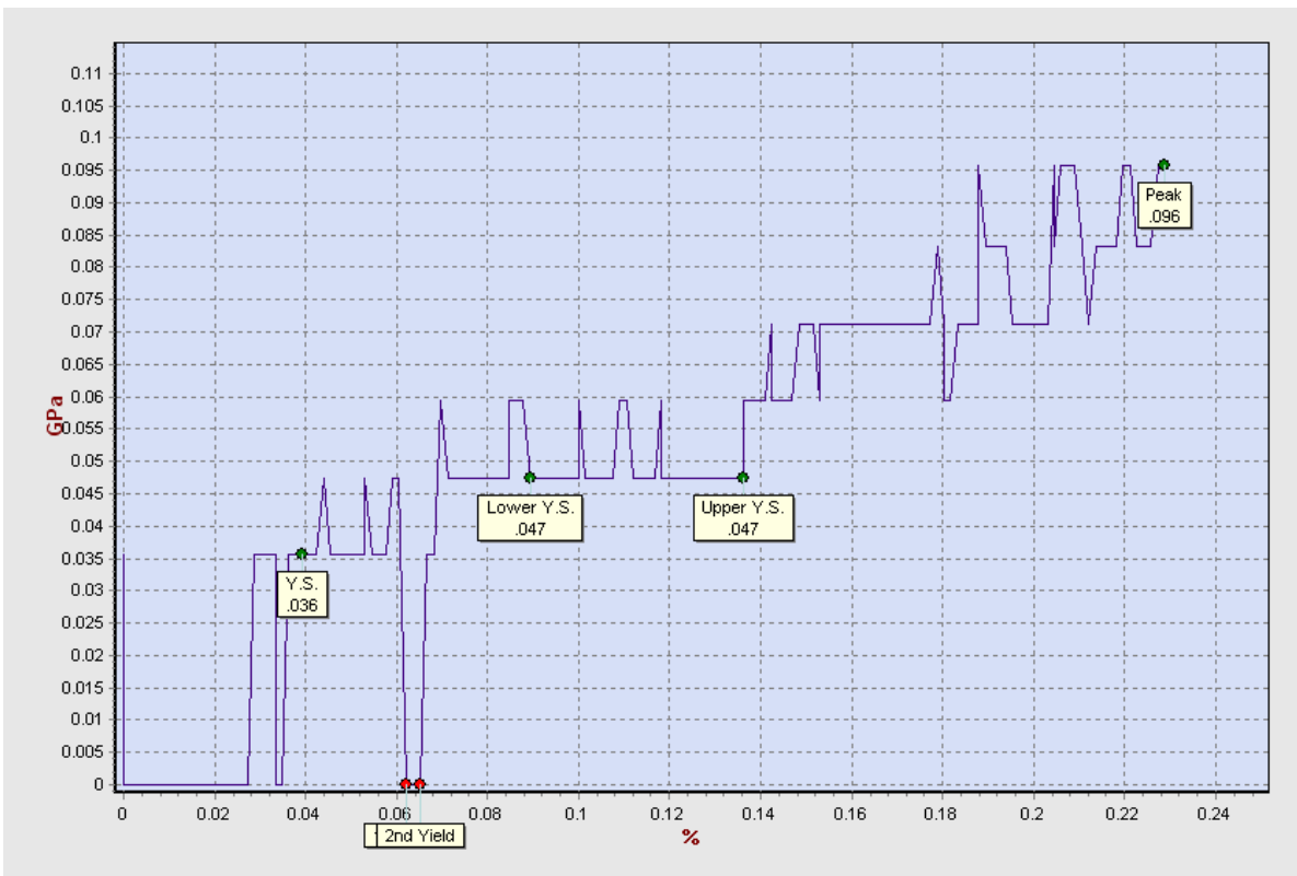
Fig.4.24 Graph showing stress value of sample subjected to 40% load of U.T.L.
