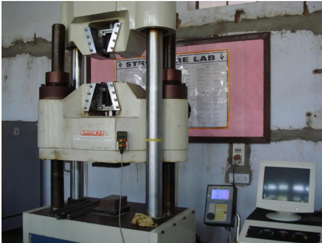
Fig. 6.1 Tensile testing machine used for testing
