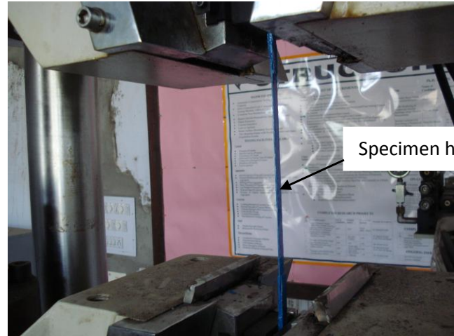
Fig. 6.2 Gripped specimen on the machine
