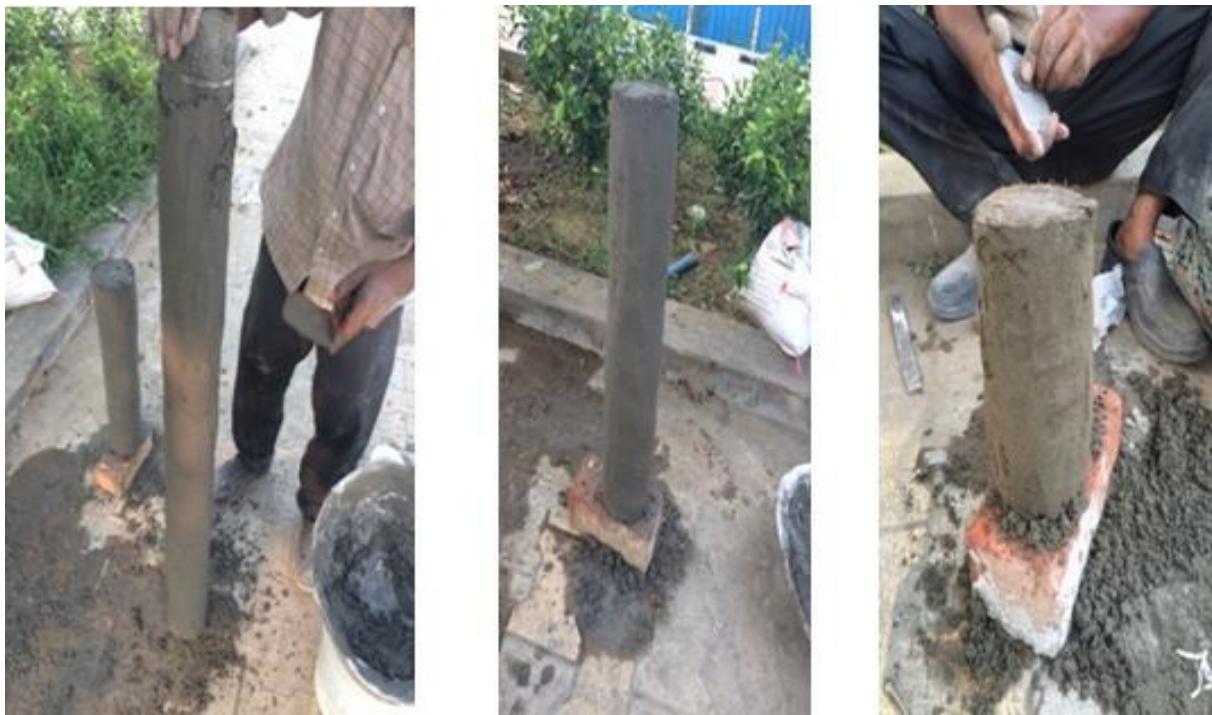
Fig. 3.4 Columns Confined with Mortar Layer
