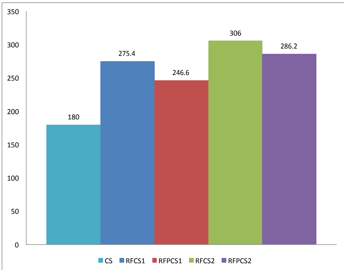
Fig. 4.22 Effect of initial damage level and no. of wire mesh on column ( \lambda=3 )
