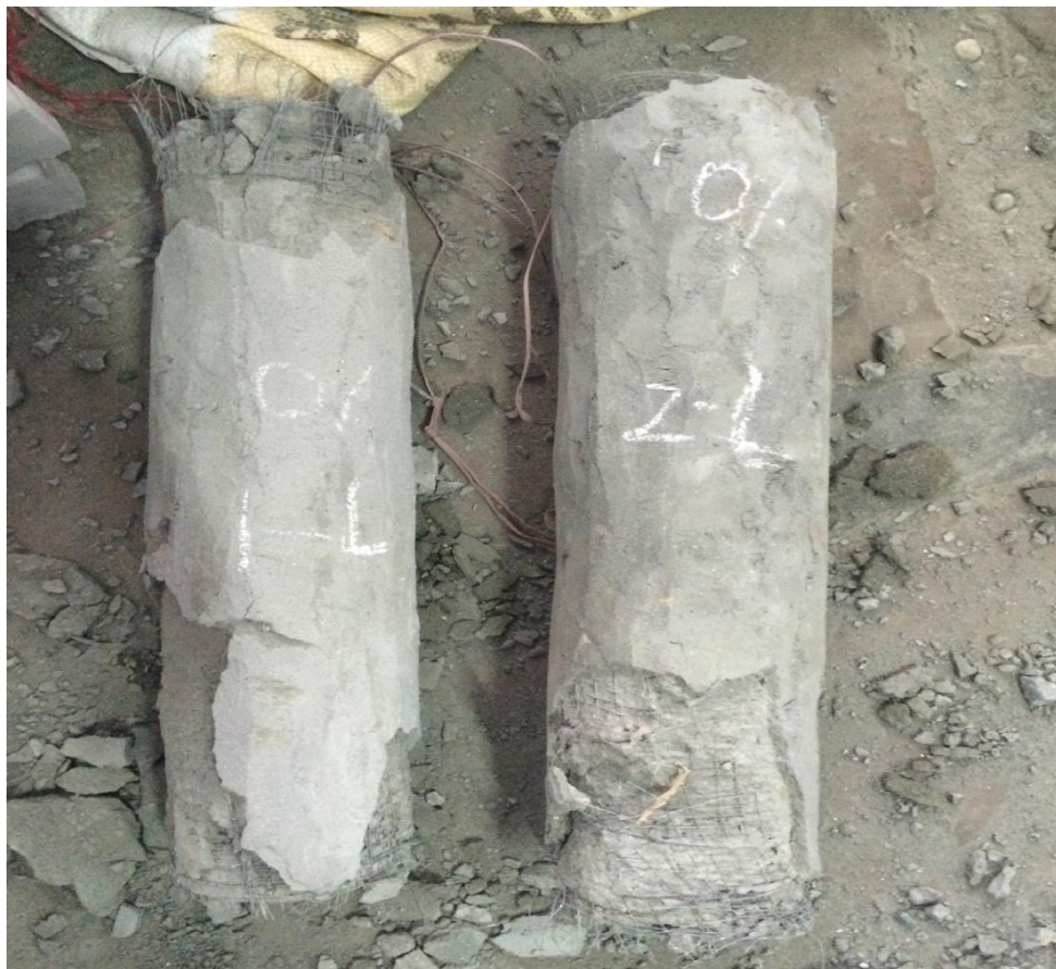
Fig. 4.11 Detail of column during final phases of loading
