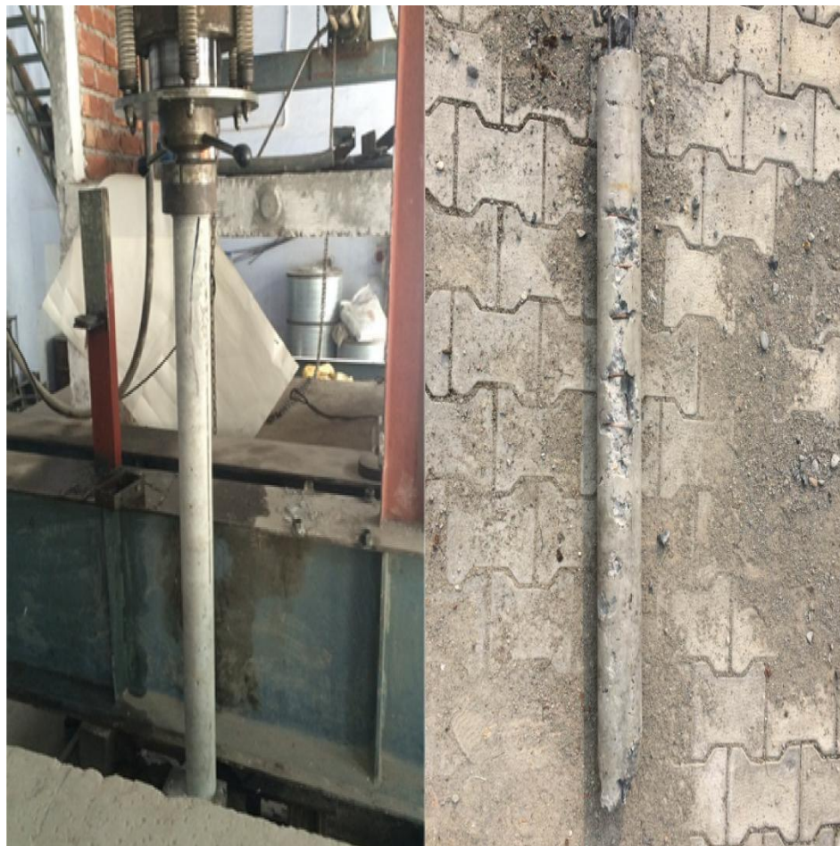
Fig. 4.16 Detail of column during final phases of loading
