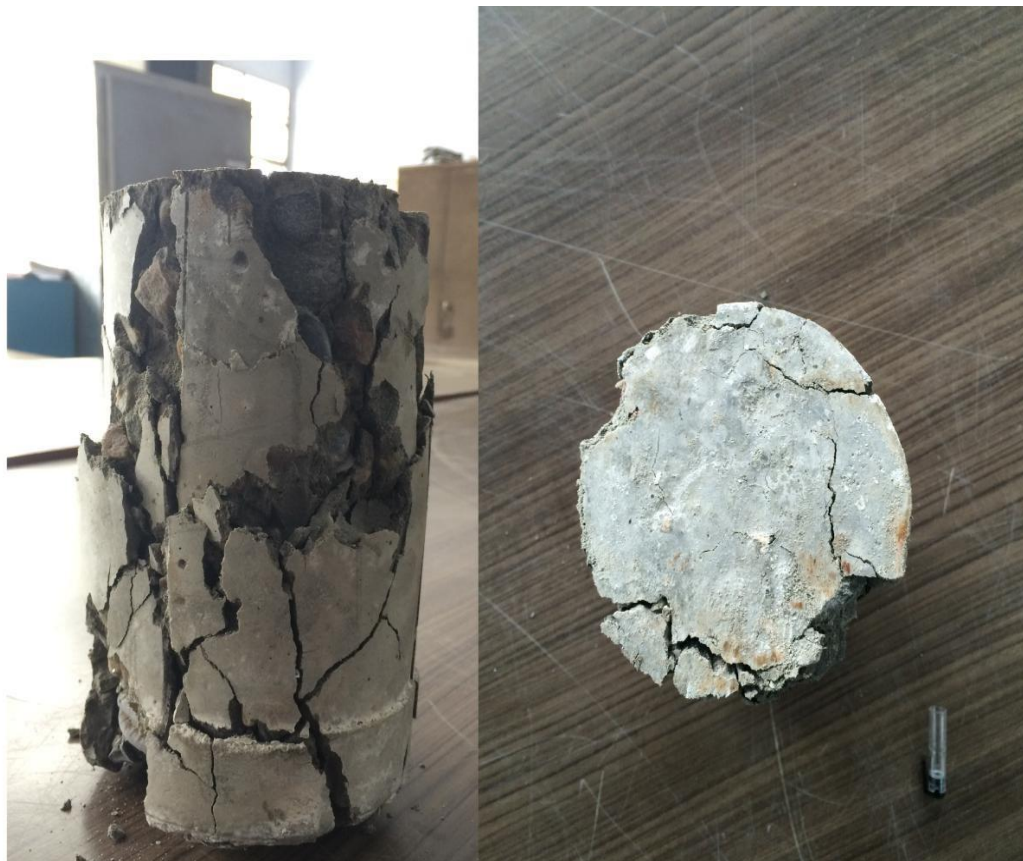
Fig. 4.2 Detail of column during initial and final phases of loading
