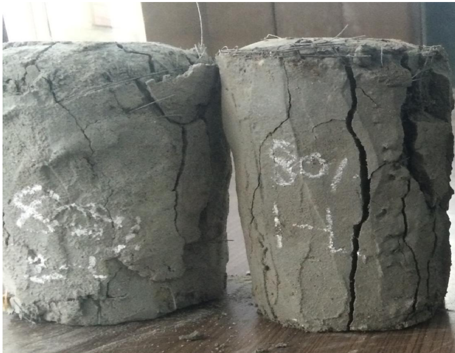
Fig. 4.6 Detail of column during final phases of loading
