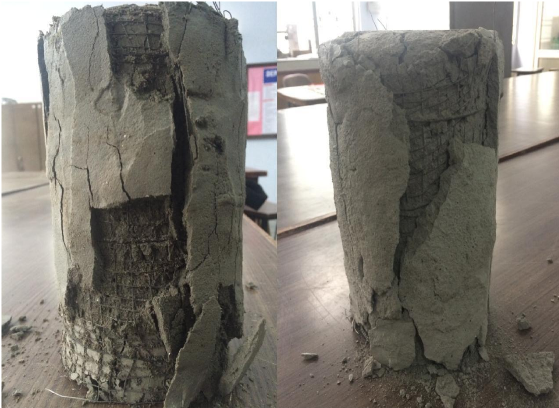
Fig. 4.4 Detail of column during final phases of loading
