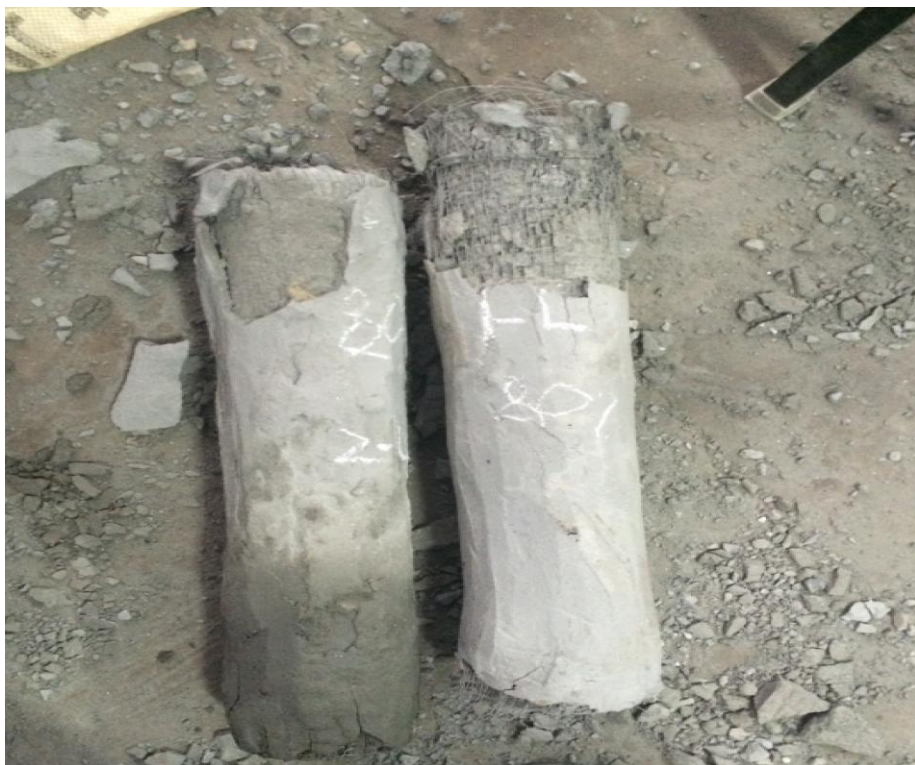
Fig. 4.13 Detail of column during final phases of loading
