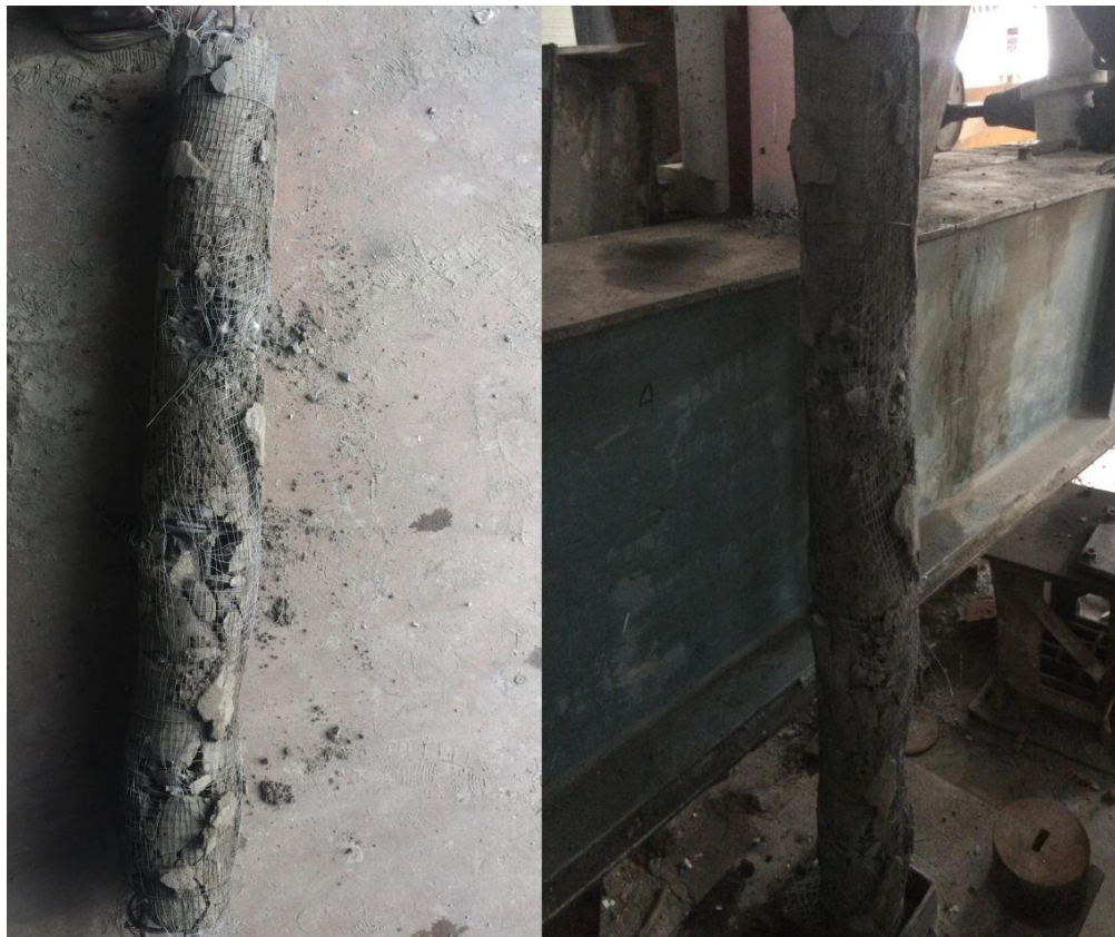
Fig. 4.18 Detail of column during final phases of loading.
