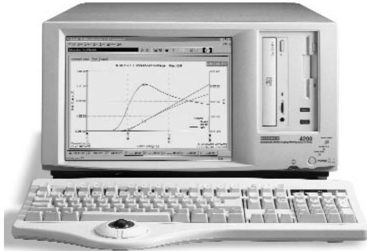
Figure-2 Two Probe System Keithley Model 4200-SCS Semiconductor Characterization system
