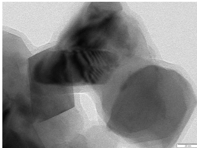
Figure 3.2: Transmission electron micrograph of manganese ferrite nanoparticles.
