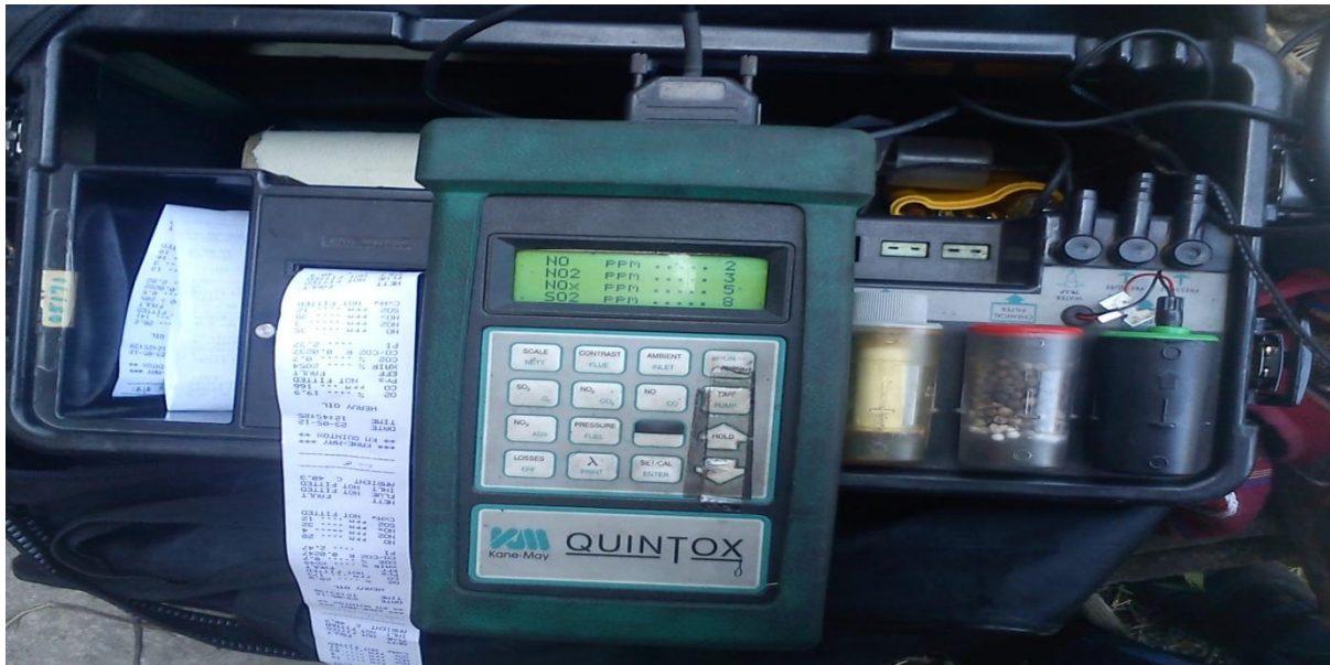
Figure 3.6 Flue gas analyzer
