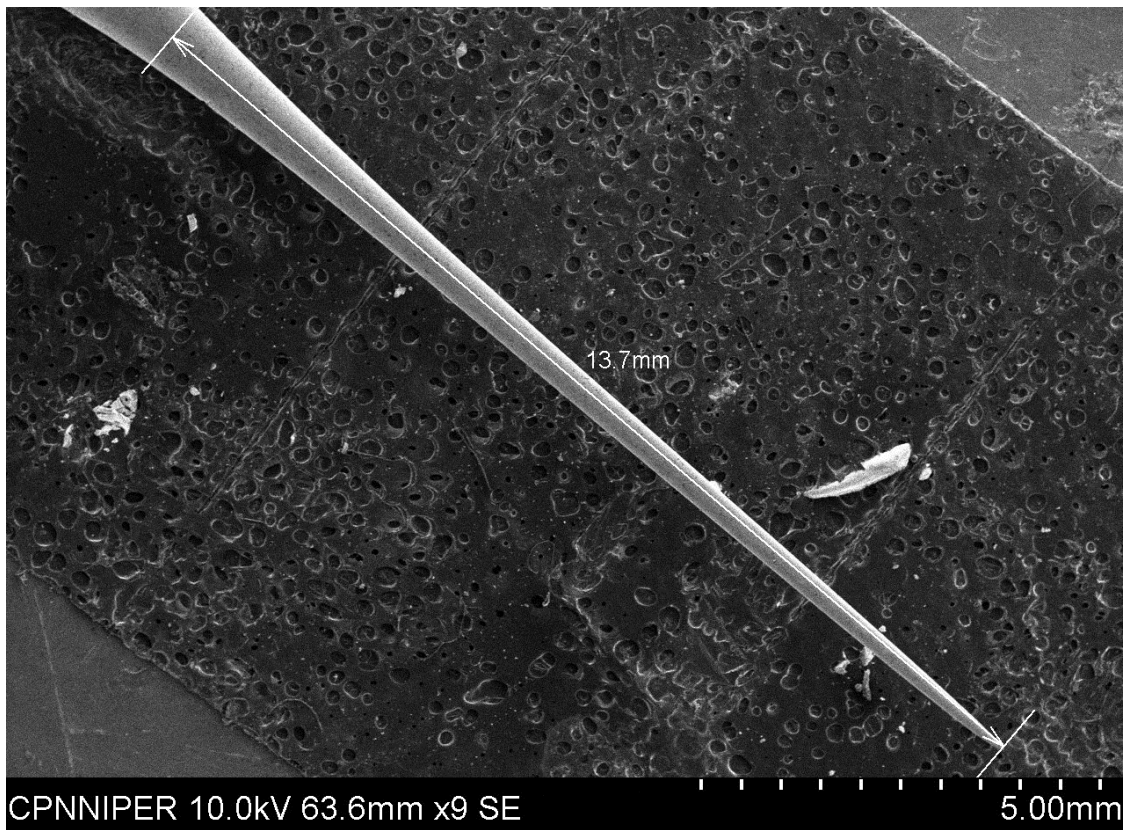
Fig 3.13 SEM View of Micro Tool after Lapping
