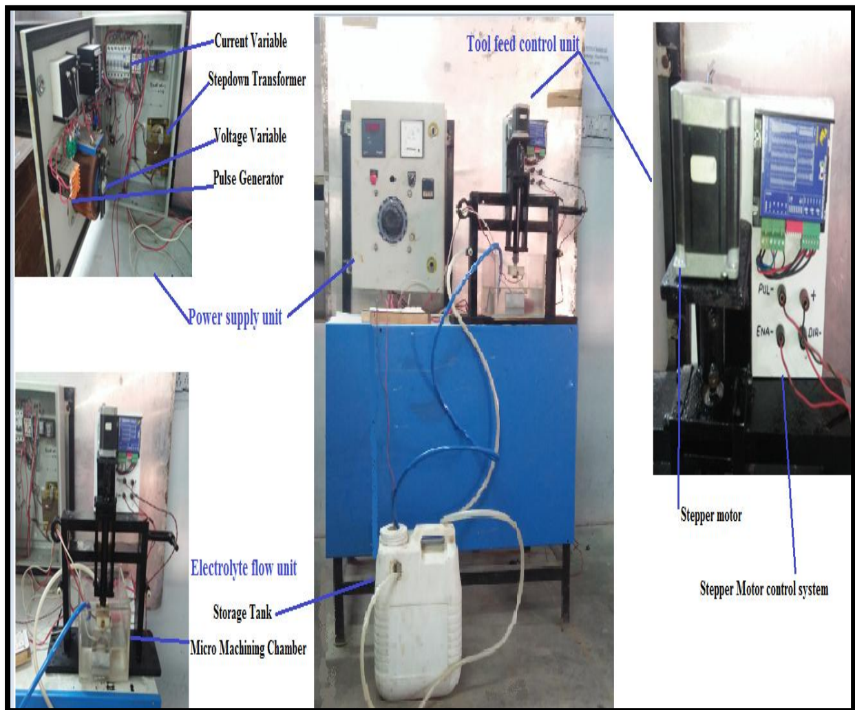
Fig. 3.2 Fabricated ECMM Setup
