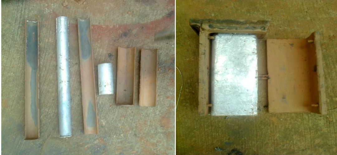
Fig. 2.9 Clay Coated Actual Mold Used with Cast MMCs
