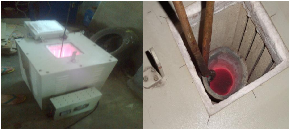
Fig. 2.6 Resistance Furnace of Capacity 1250°C Used for Pre-Heating of Reinforced Particles ( \text{Al}_2\text{O}_3 , SiC, and C)
