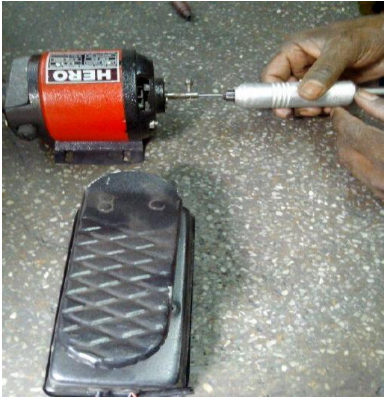
Fig 3.8 A View of Fabricated Micro Grinding Setup
