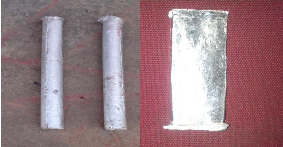
Fig. 2.10 Cast MMCs Specimens
