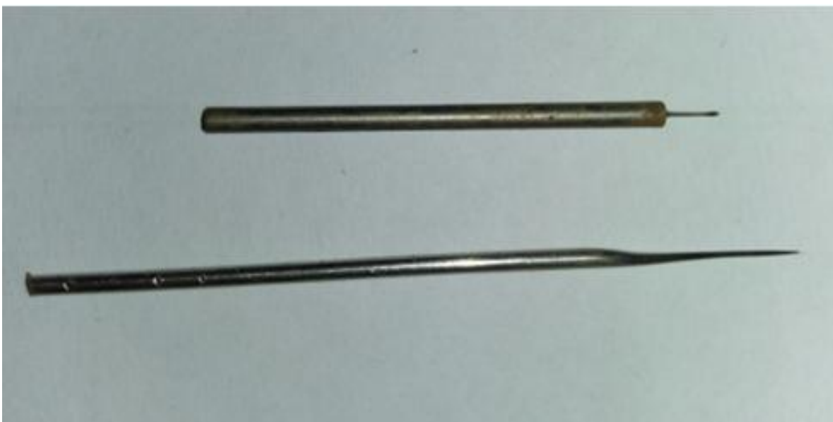
Fig 3.9 Fabricated Tungsten Micro Tool
