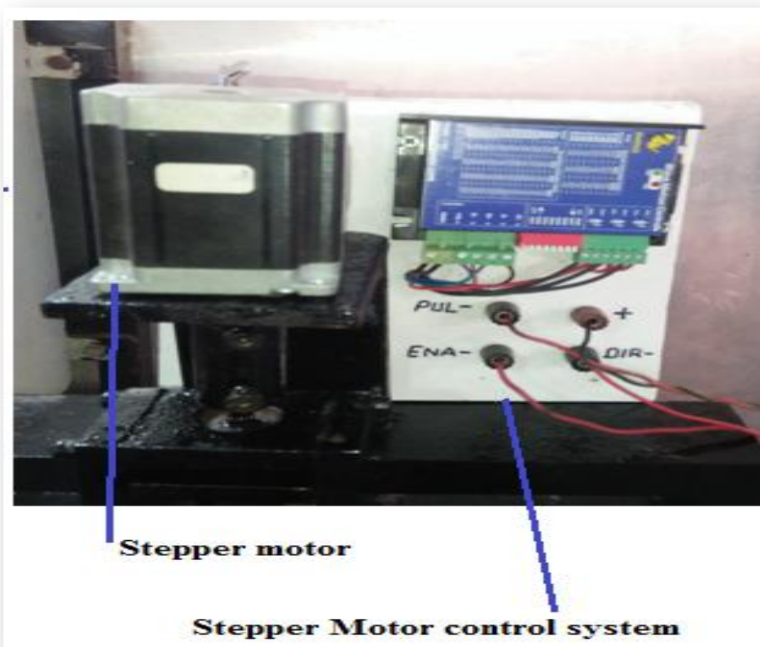
Fig. 3.6 Servo Control and Feed Unit
