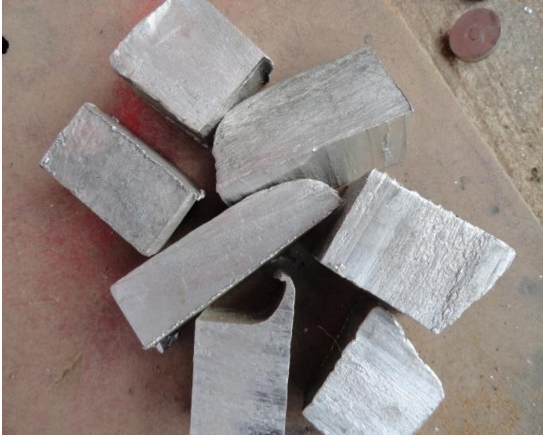
Fig. 2.1 Pure Aluminum Pieces for Matrix Metal
