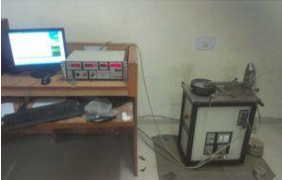
Fig. 1.4 Pin on Disc Machine Setup [Tribology Lab MMU]
