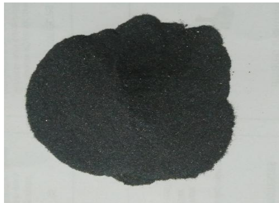
Fig. 2.3 SiC Reinforced Particulates
