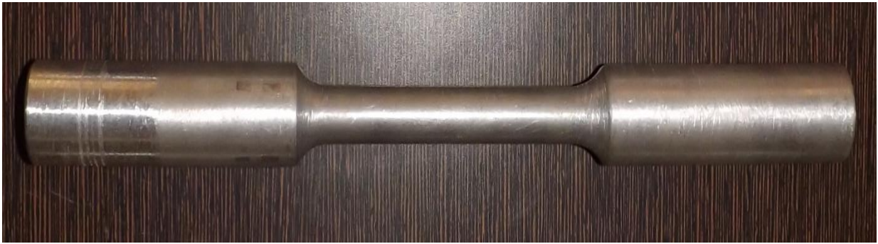
Fig. 2.15 Tensile Strength Test Specimen
