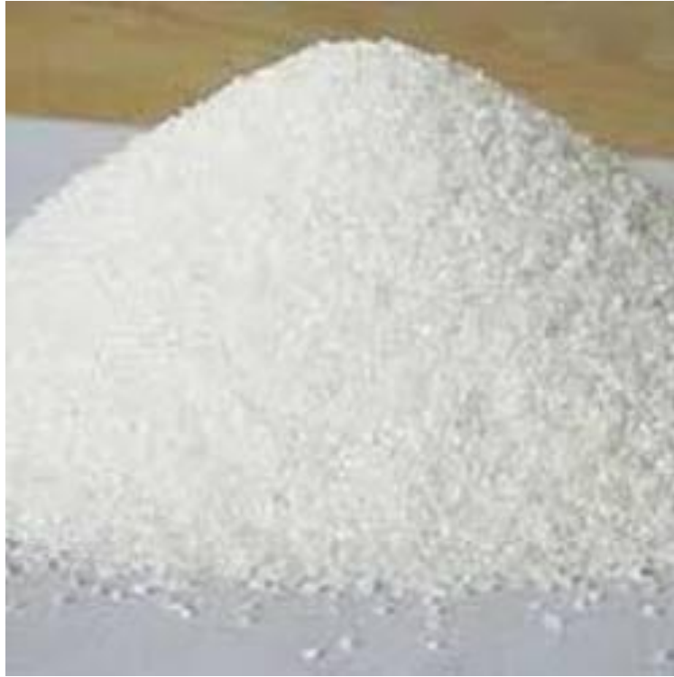
Fig. 2.2 Al 2 O 3 Reinforced Particulates
