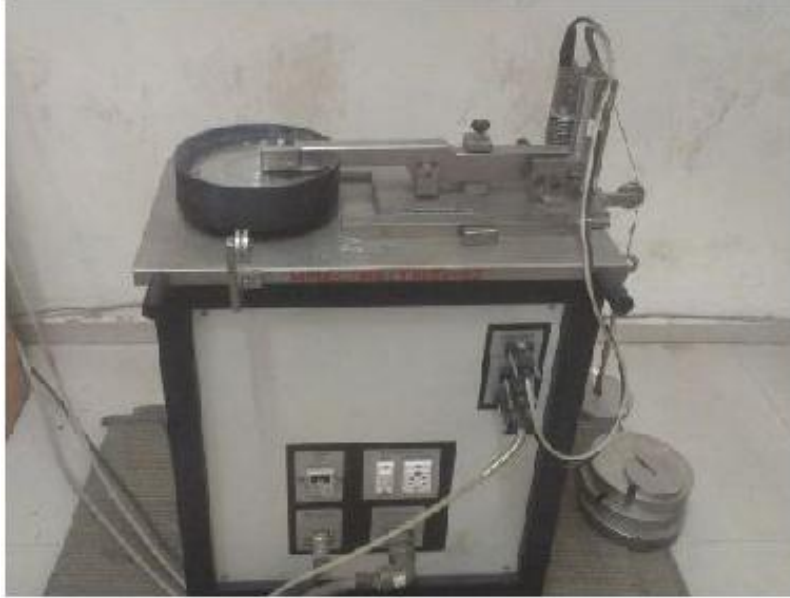
Fig 2.29 Pin on Disc Machine used for Wear Test of MMC and Hybrid MMC Specimens
