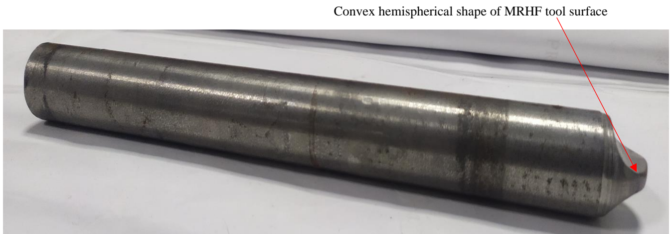
Fig. 3.26 Fabricated magnetorheological hemispherical finishing tool core for finishing the blind hole type ball cup workpiece surface.
