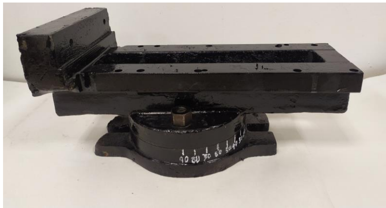
Fig. 3.22 Swivel vise for maintaining uniform working gap during finishing of the internal tapered longitudinal surface using the magnetorheological grinding tool.
