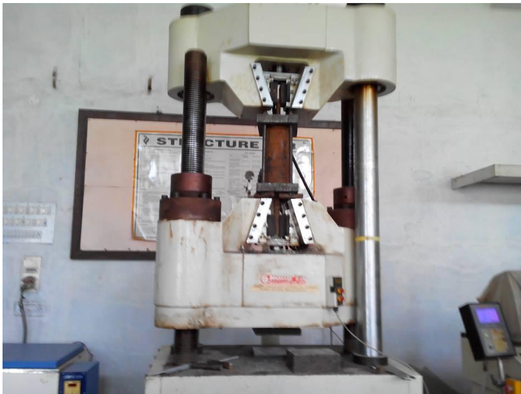
Fig. 5.13: Pull-out test set-up
