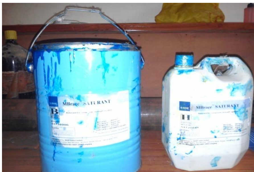
Fig. 4.4: Adhesive used for bonding FRP with concrete
