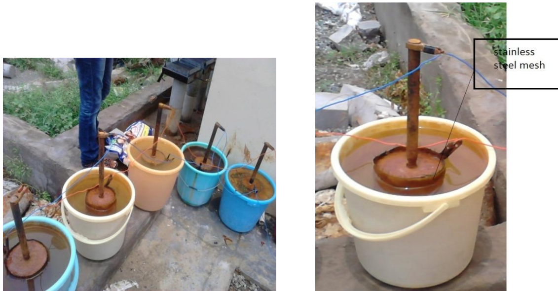
Fig. 4.5: (a) Cylindrical Specimens (b) Specimen wrapped with stainless steel
