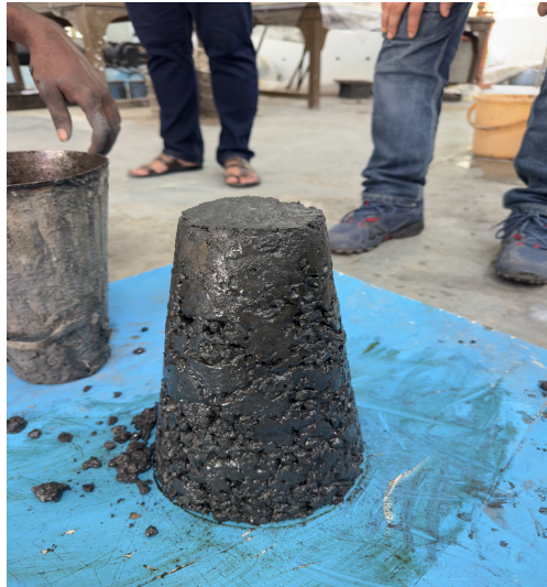
Figure 3.5 Slump cone test
