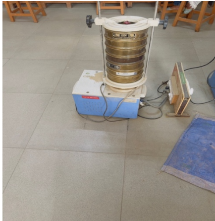
Figure 3.1 Mechanical sieve shaker used for sieve analysis of fine aggregate
