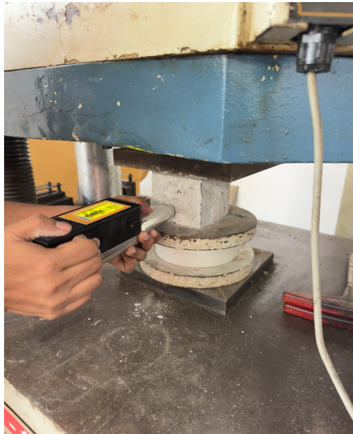
Figure 3.6 Rebound hammer test
