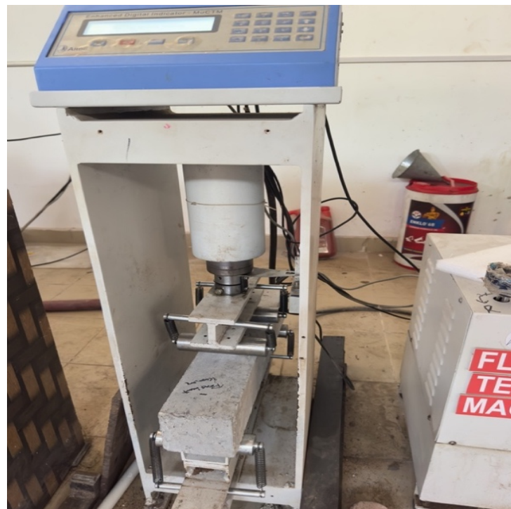
Figure 3.10 Flexural strength test set-up
