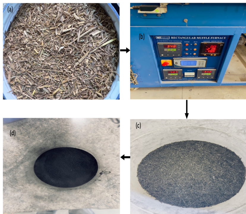
Figure 3.3 Different stages of biochar production
