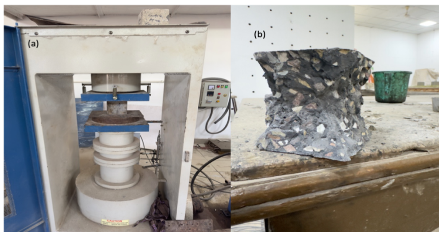
Figure 3.8 (a) Compressive strength test (b) Compression failure pattern
