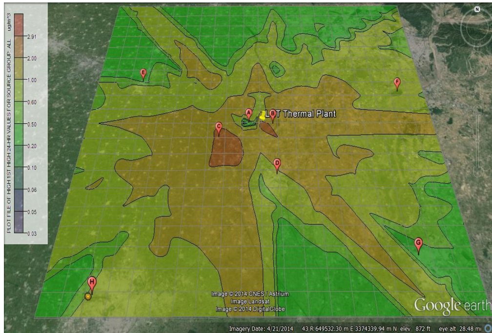
Figure 5.17 ISCST3 daily average ground level concentrations ( \mu\text{g}/\text{m}^3 ) of SPM due to power plant
