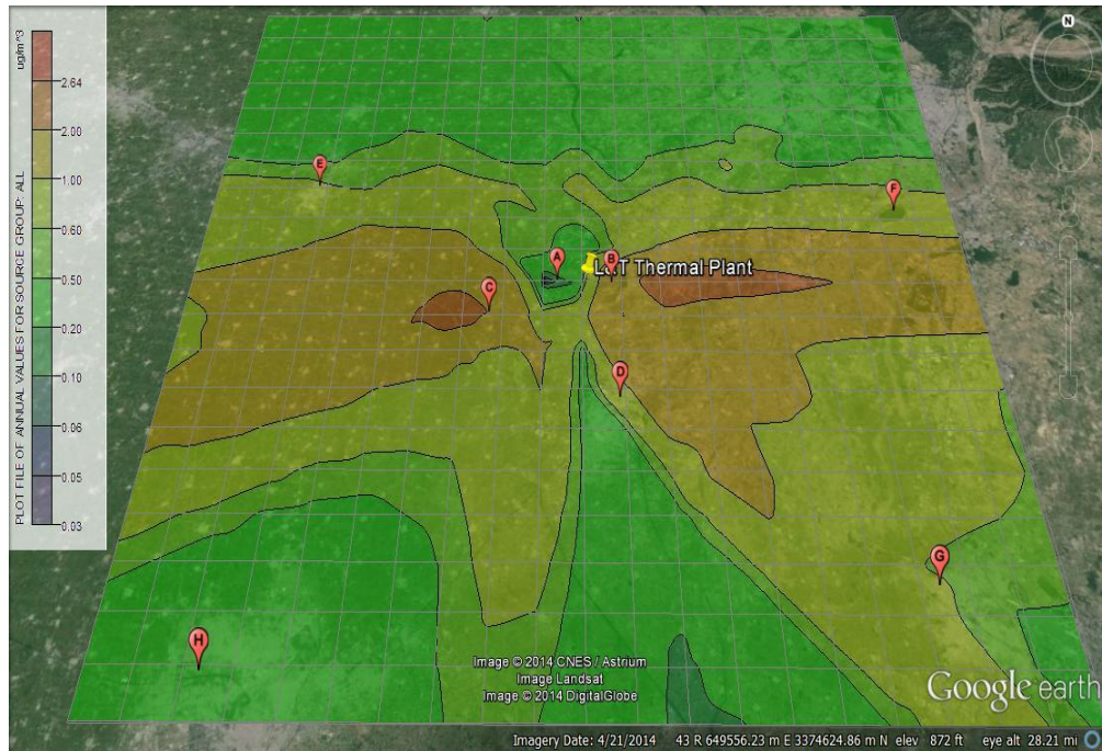
Figure 5.11 ISCST3 annual average ground level concentrations ( \mu\text{g}/\text{m}^3 ) of \text{SO}_2 due to power plant
