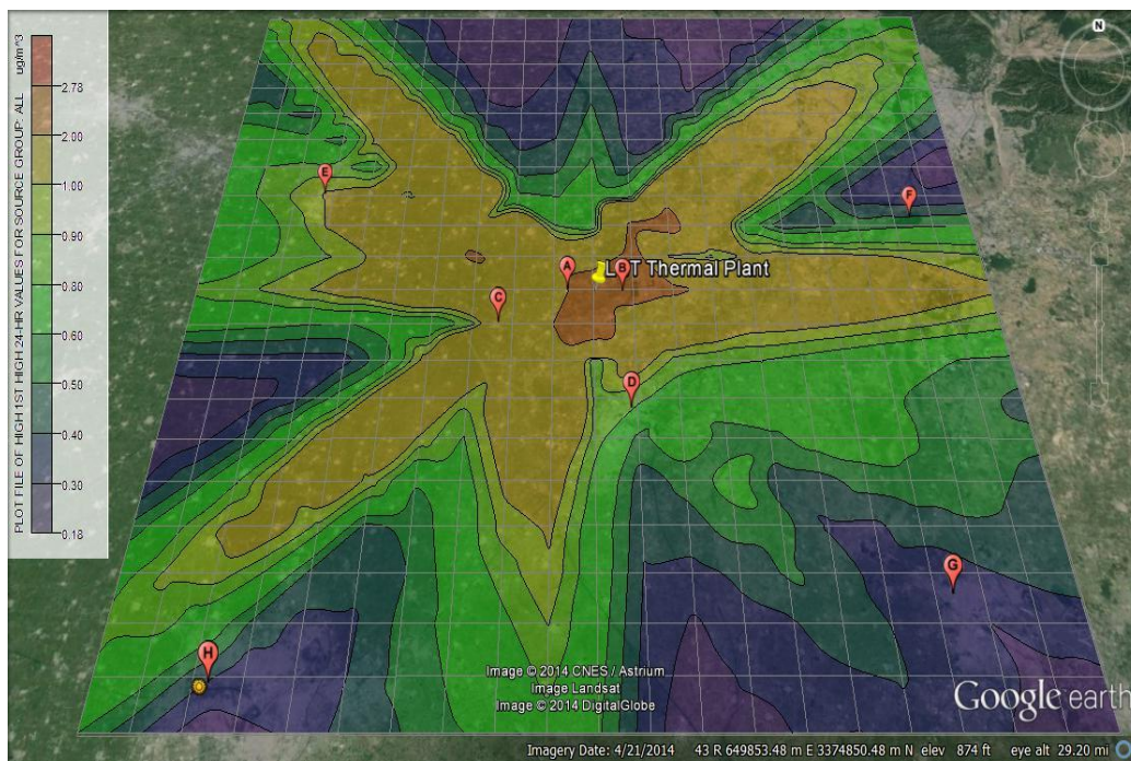
Figure 5.18 AERMOD daily average ground level concentrations ( \mu\text{g}/\text{m}^3 ) of SPM due to power plant
