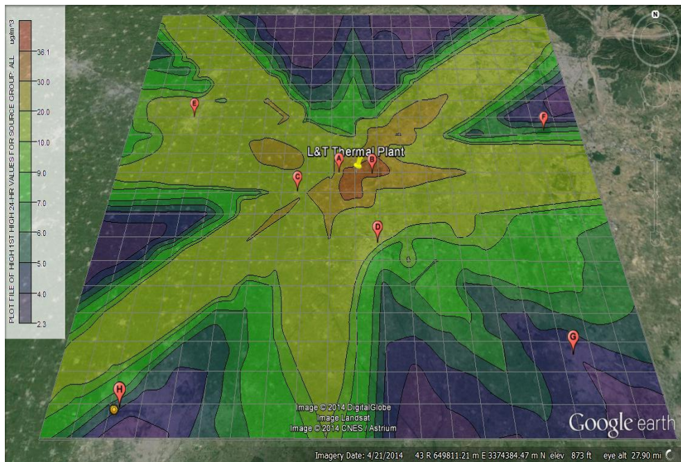
Figure 5.10 AERMOD daily average ground level concentrations ( \mu\text{g}/\text{m}^3 ) of NO 2 due to power plant
