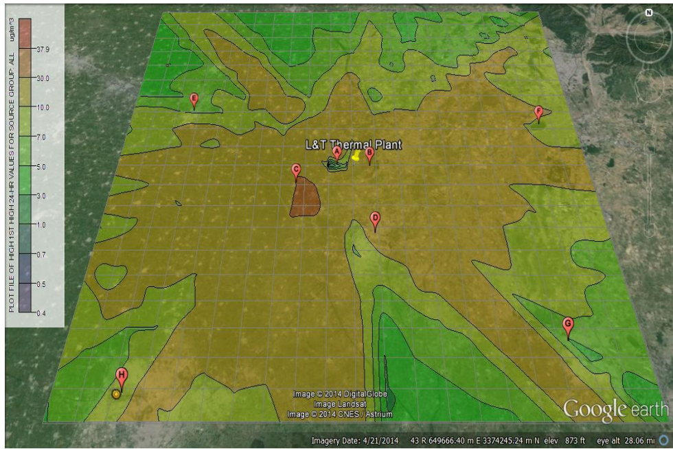
Figure 5.9 ISCST3 daily average ground level concentrations ( \mu\text{g}/\text{m}^3 ) of NO 2 due to power plant
