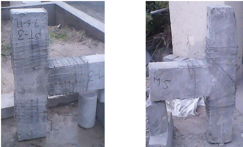
Figure 2. 5 Specimen Retrofitted with Mesh Wire (Scheme I and Scheme II) (Bansal et al., 2016).
