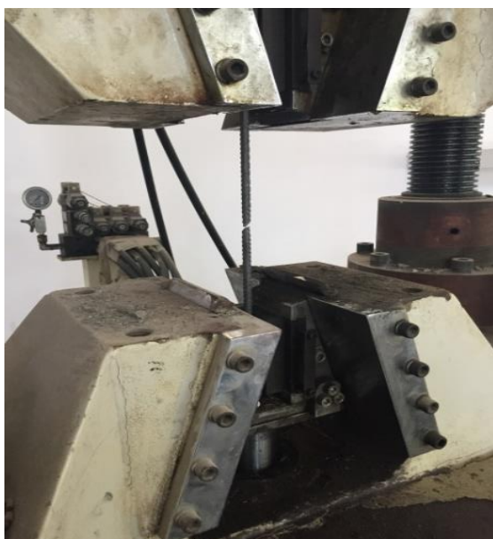
a) Breaking of Reinforcement
