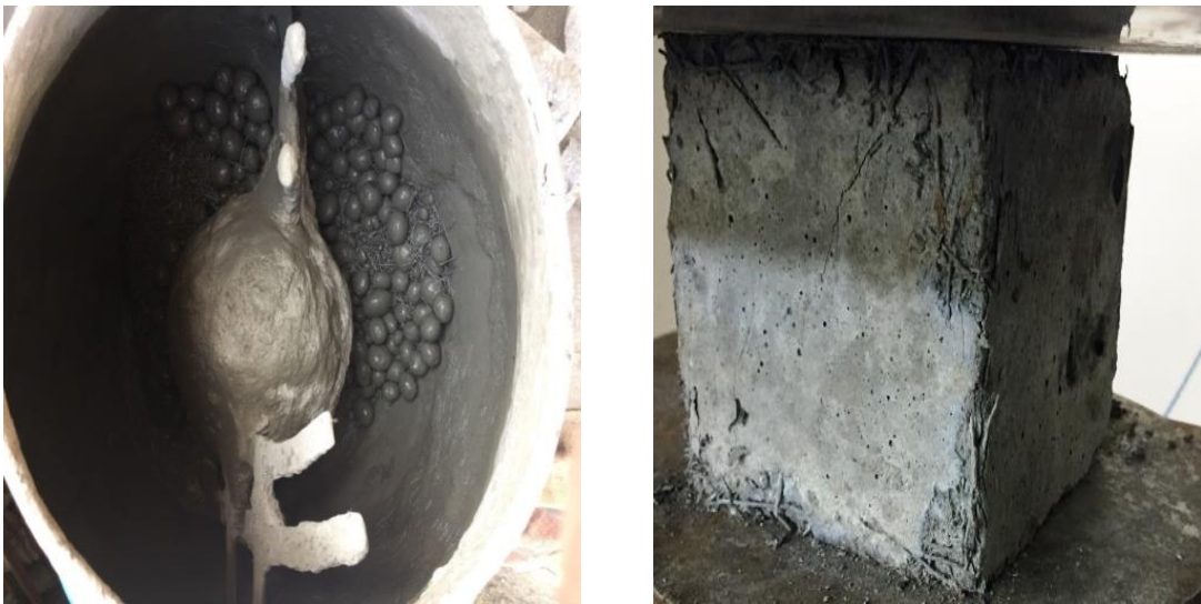
Figure 3. 13. Balling effect during mixing of mortar in the mixer and Bundling of fibers
