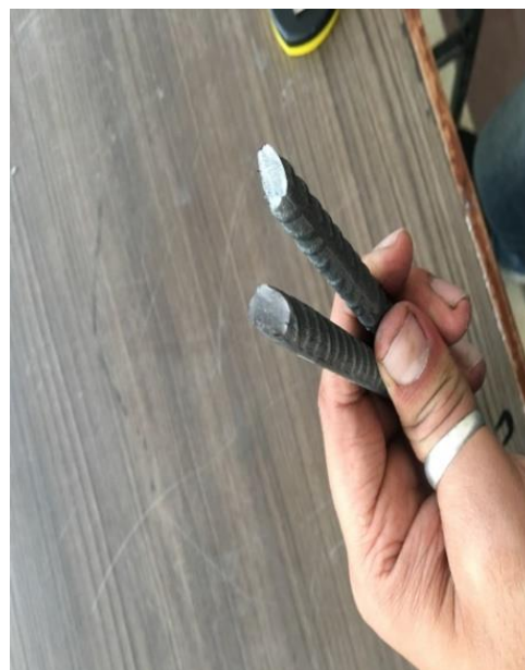
b) Fracture of Reinforcement at 45°
