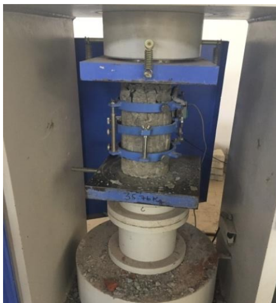
Figure 3. 8 Testing of Cylinder on CTM to calculate stress strain graph
