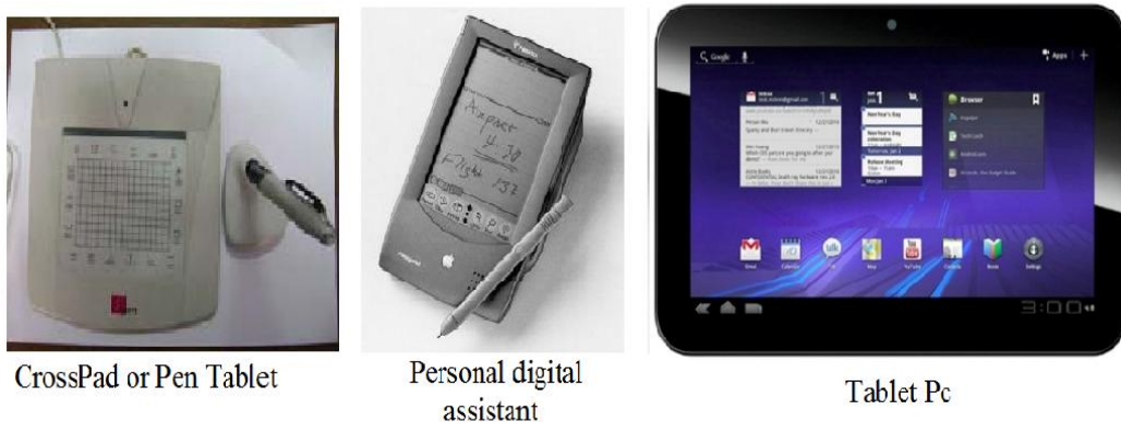
Fig. 2.2: Commonly used hardware devices for capturing handwriting.
