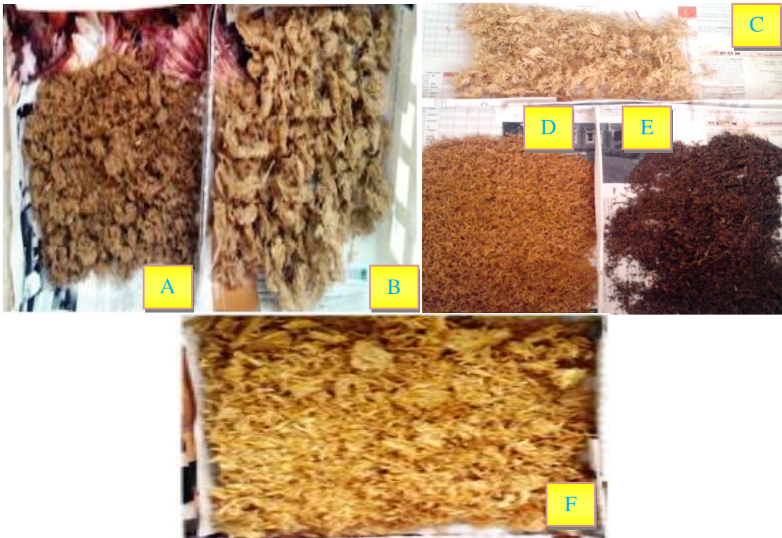
Fig 5. Alkali treated Agro-wastes : Bamboo leaves(A), Rice straw(b), Bagasse(C), Rice bran(D), Eucalyptus leaves(E), Wheat straw(F).
