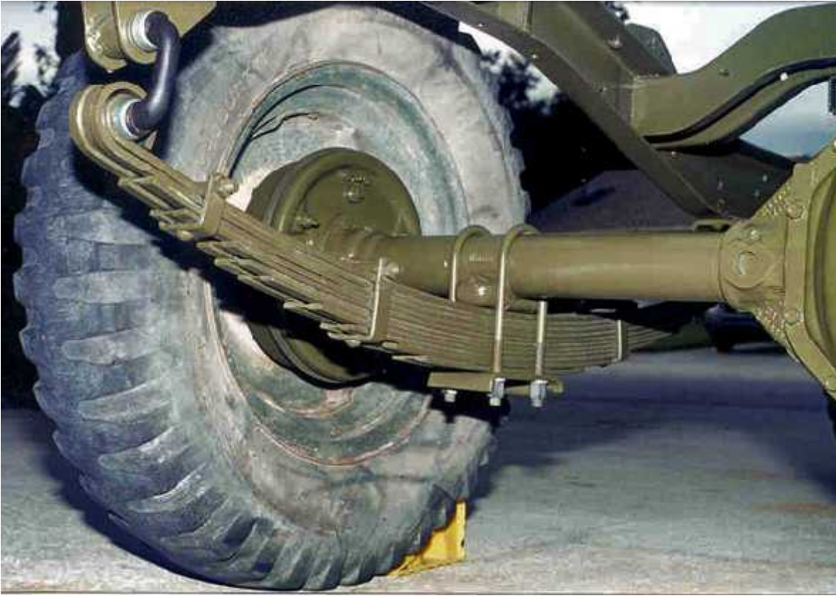
Figure 1.1: Leaf spring assembled at rear axle of automotive [1]
