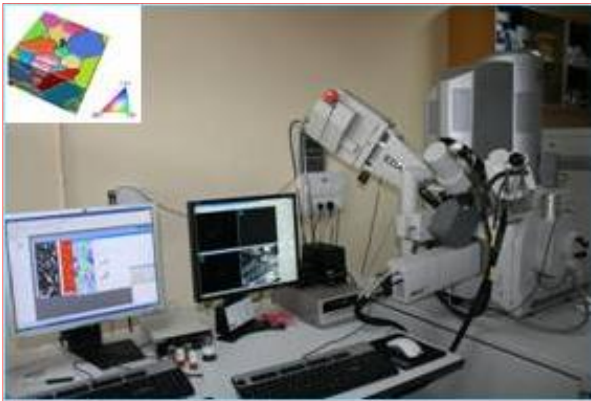
Figure 4.5 3D Electron Back Scattered Diffraction by Field Emission Gun (Make: JEOL; Model: JSM- 7600F; Japan) (Courtesy: National Facility Orientation Imaging Microscopy & X-Ray Bulk Texture, IIT Bombay)
