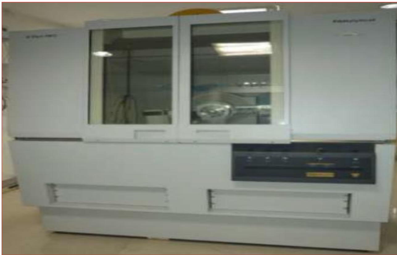
Fig 4.6 X-Ray Diffractometer (Make: PANalytical; Model: X'Pert Pro; Netherland) (Courtesy: SAI Labs, Thapar Institute of Engineering and Technology, Patiala)
