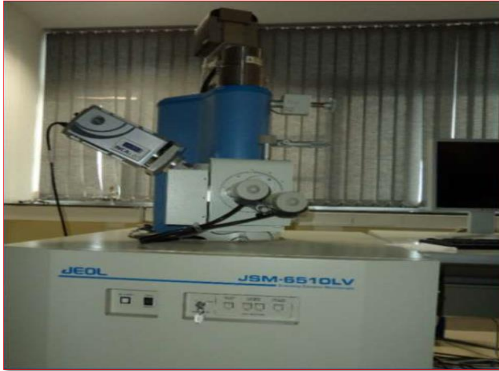
Figure 4.4 Scanning Electron Microscopy (Make: JEOL; Model: JSM- 6510LV; Japan) (Courtesy: SAI Labs, Thapar Institute of Engineering and Technology, Patiala)
