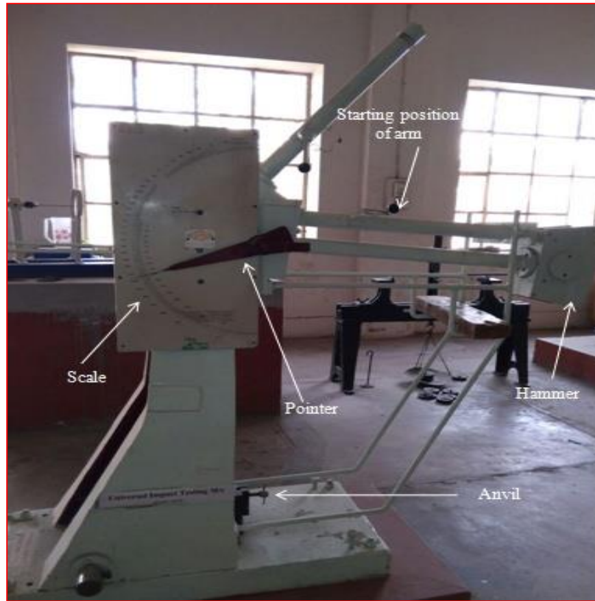
Figure 4.10 Impact Testing Machine (Courtesy: Solid Mechanics lab, Thapar Institute of Engineering & Technology, Patiala)
