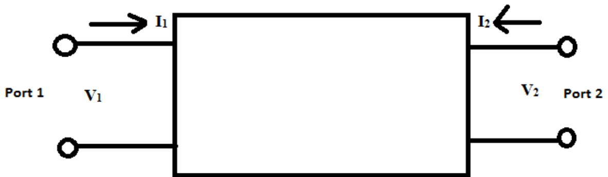
Figure 2.17: 2 port network of transmission line.
