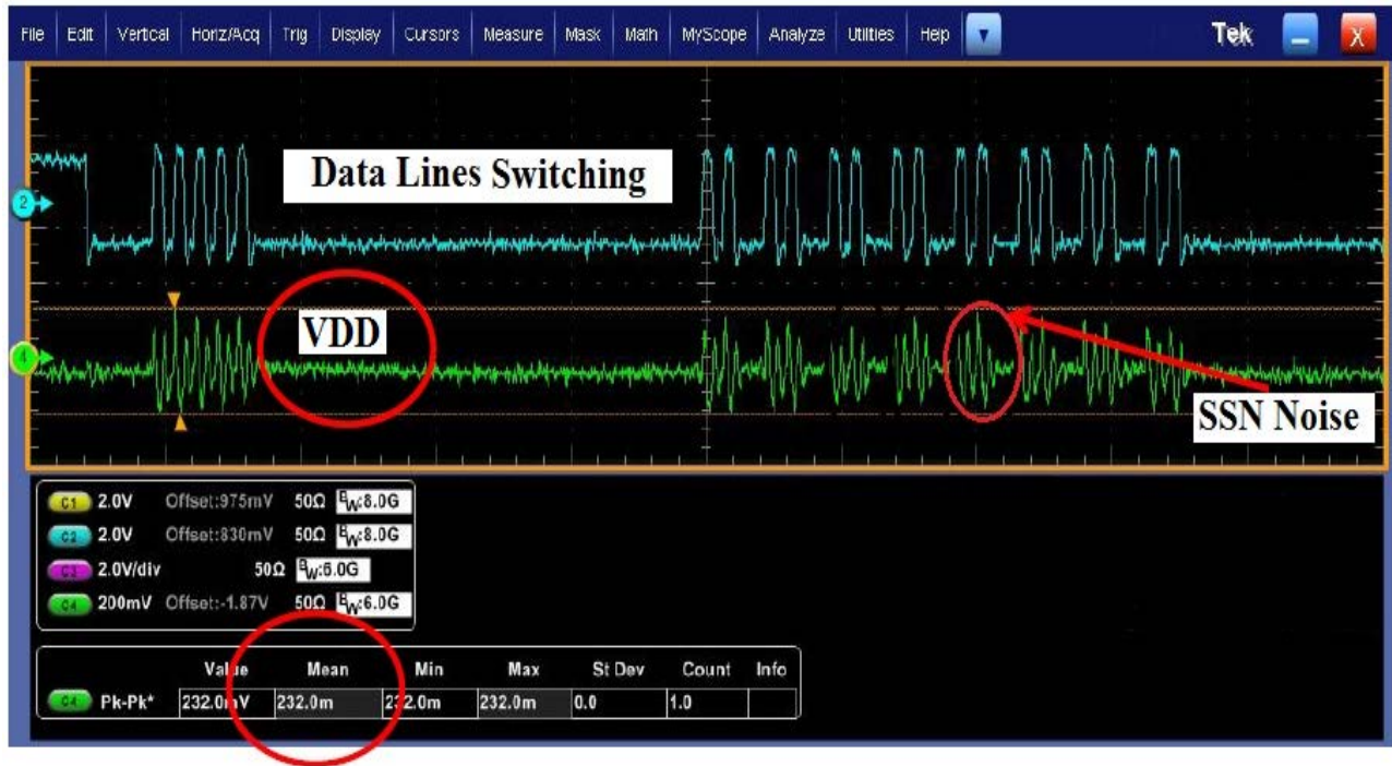
Figure 6.12: SSN noise in 6 layer structure board.
