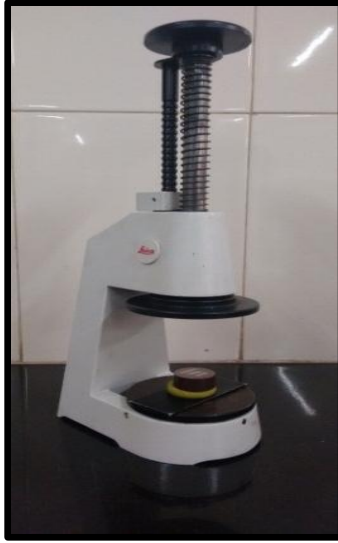
Figure 3.6: Leveling machine (Courtesy: NML, Jamshedpur)
