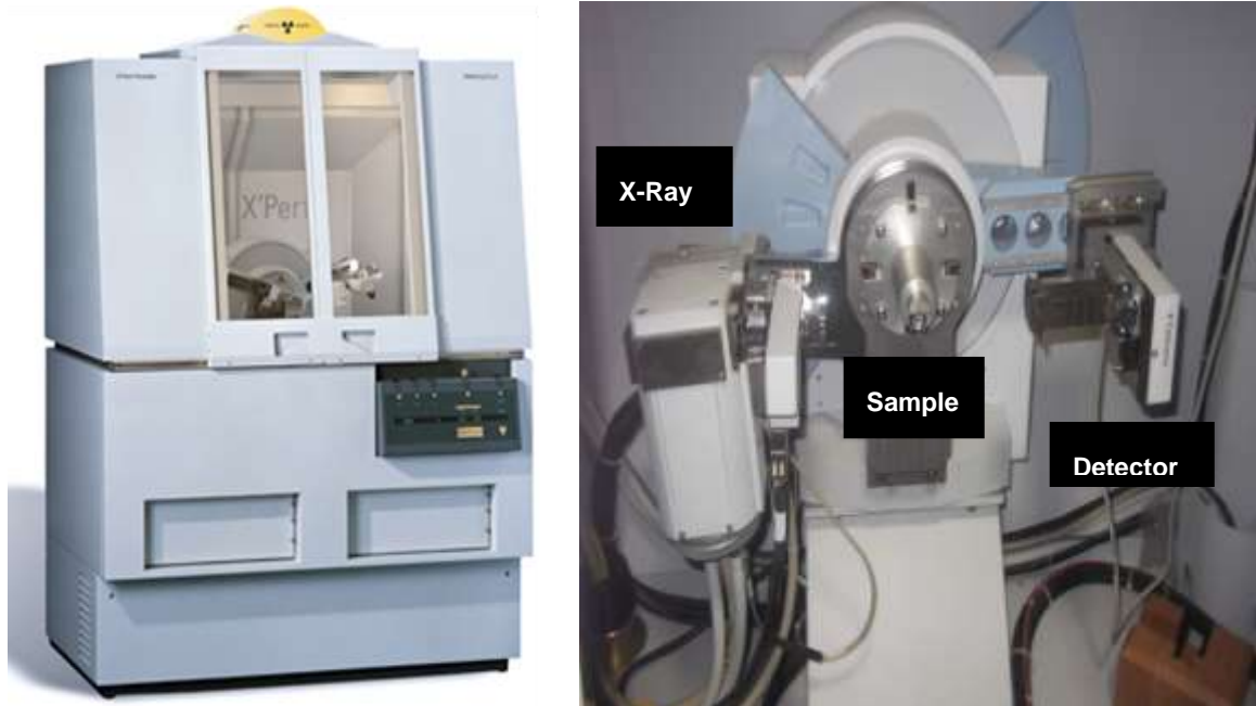
Figure E.1 XRD machine used for the residual stress measurements
