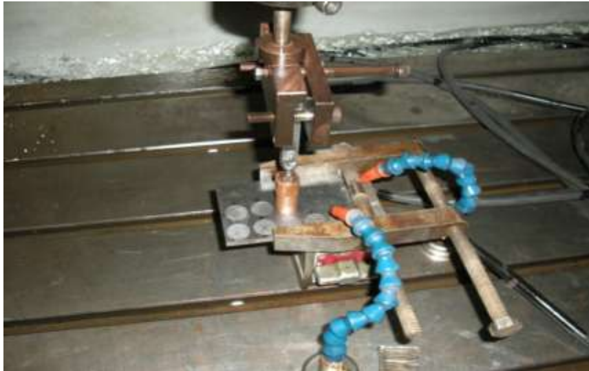
Figure C.3 Tool and workpiece set-up in EDM process
