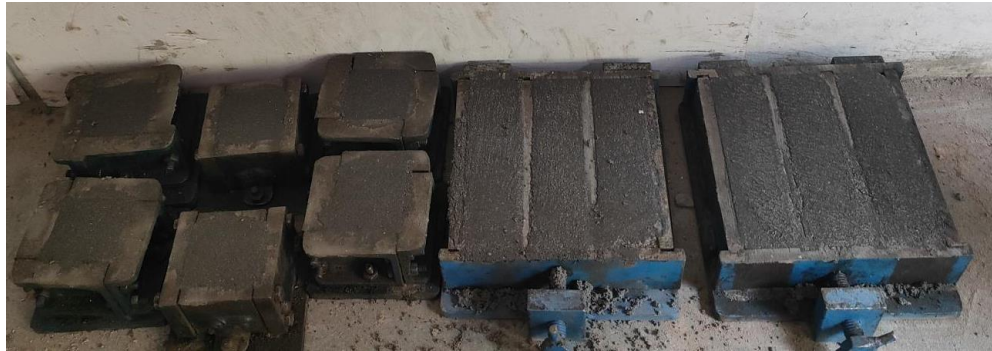
Figure 3.30 Casting of Cubical and Prism Moulds
