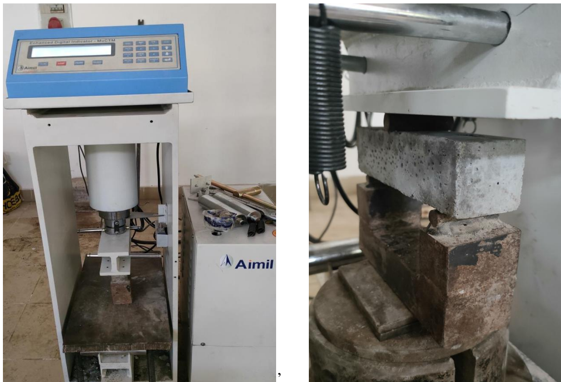
Figure 3.38 Flexural Testing Machine for determining Flexural Strength
