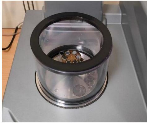
Figure 3.13 Gold plating on the Lead slag (SAI Lab, Thapar University)
