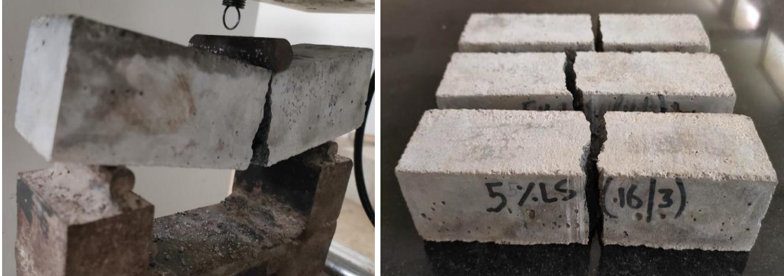
Figure 3.40 Specimens after 3 point load test
