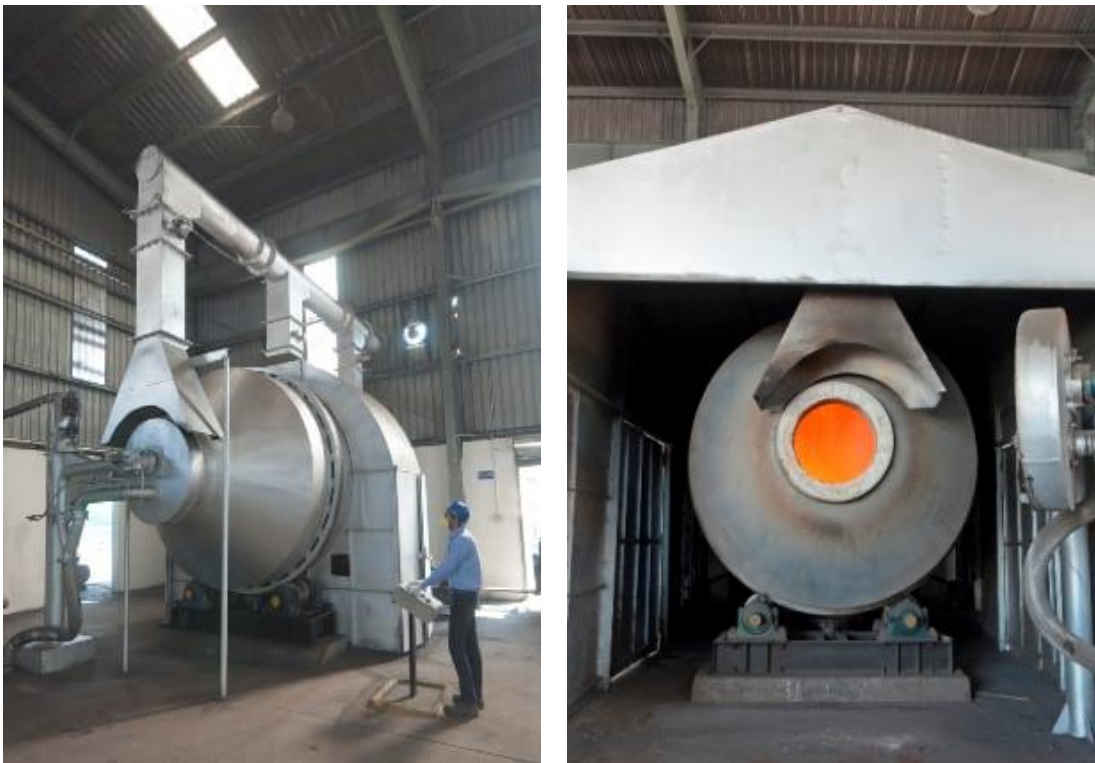
Figure 3.6 Rotary Furnace for Lead Battery Recycling (Recycling Plant)
