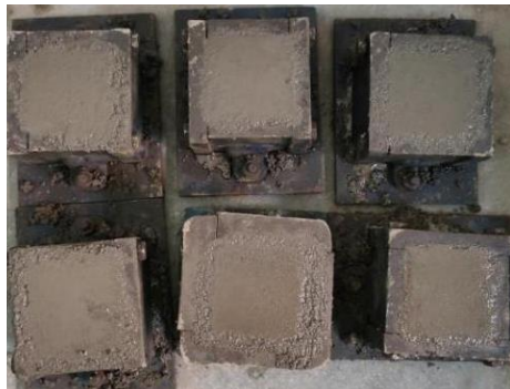
Figure 3.33 Casting of Cubical Moulds
