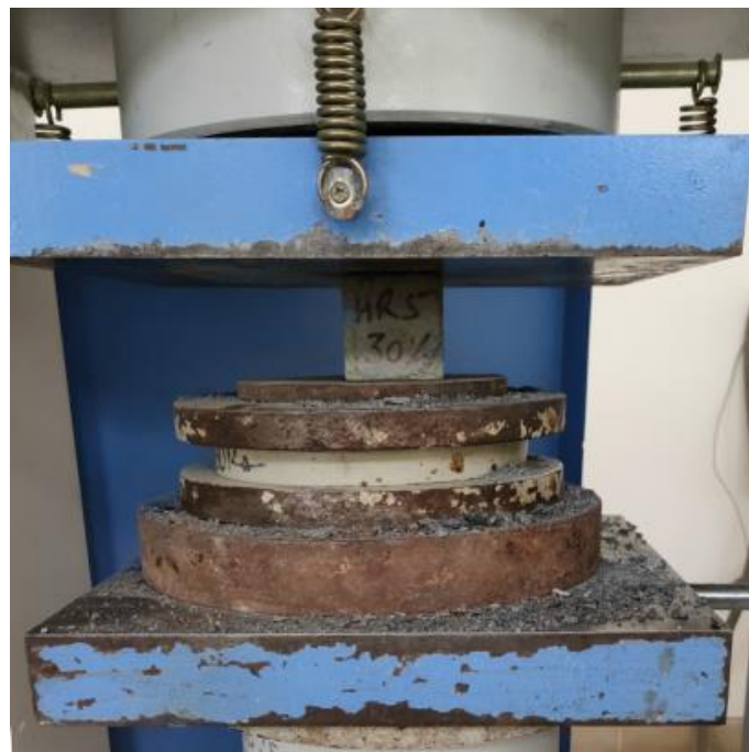
Figure 3.37 CTM for Compression Strength Test
