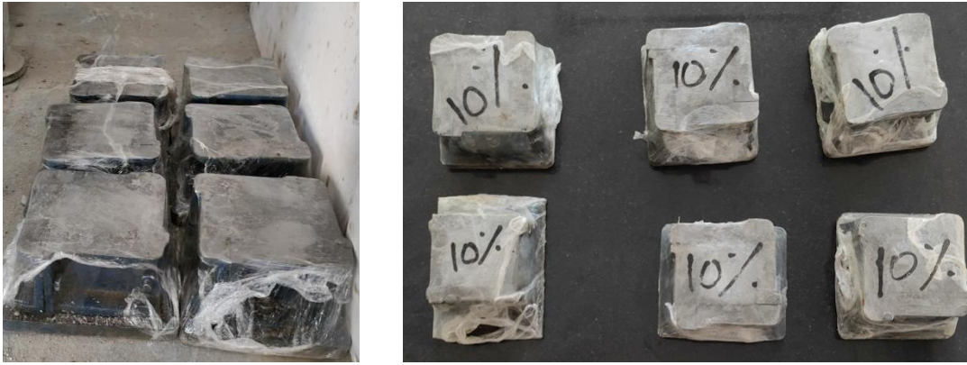
Figure 3.34 Mould wrapped with a thin film of plastic polythene
