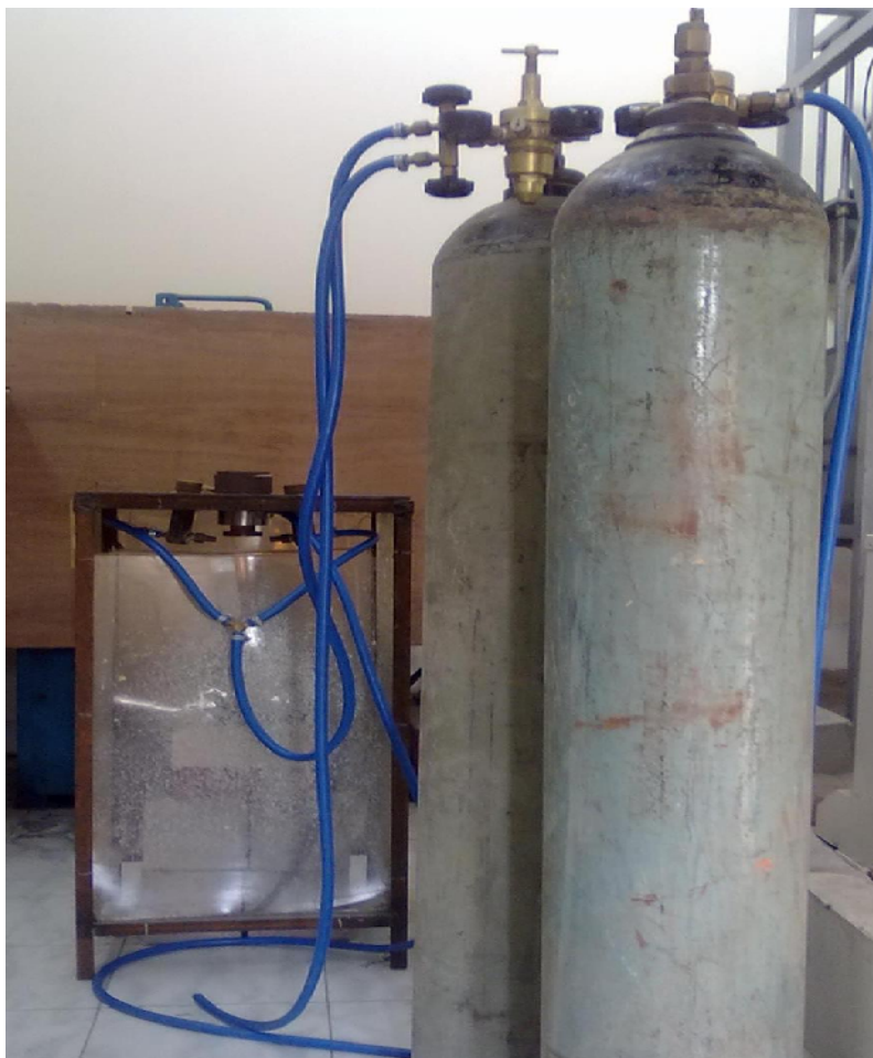
Fig. 4.1: Spray casting set up.
