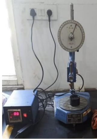
Figure 22. Penetration test equipment
