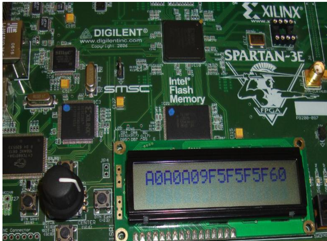
Figure 6.2: LCD Display of 32-bit Booth Wallace MAC Unit
