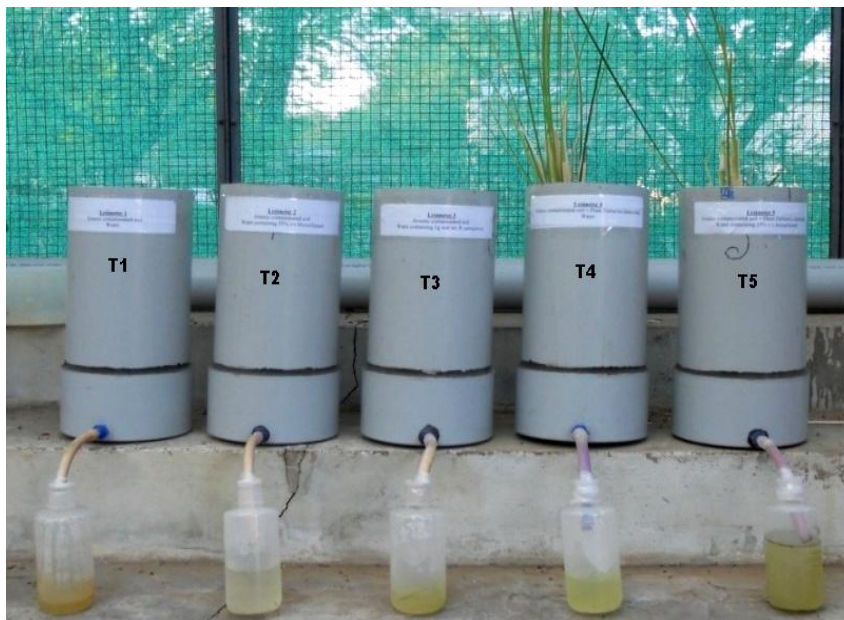
Fig 2: Lysimeter studies for arsenic removal
