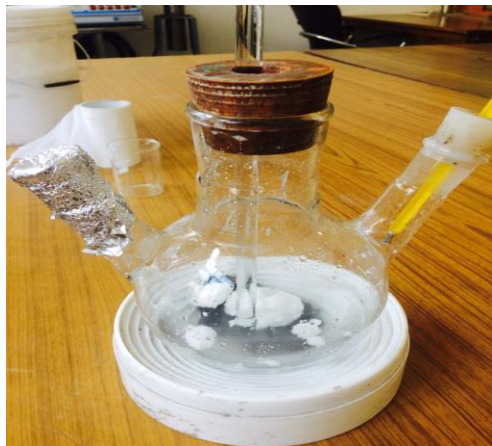
Figure 3.2 Coagulation of PVAc
