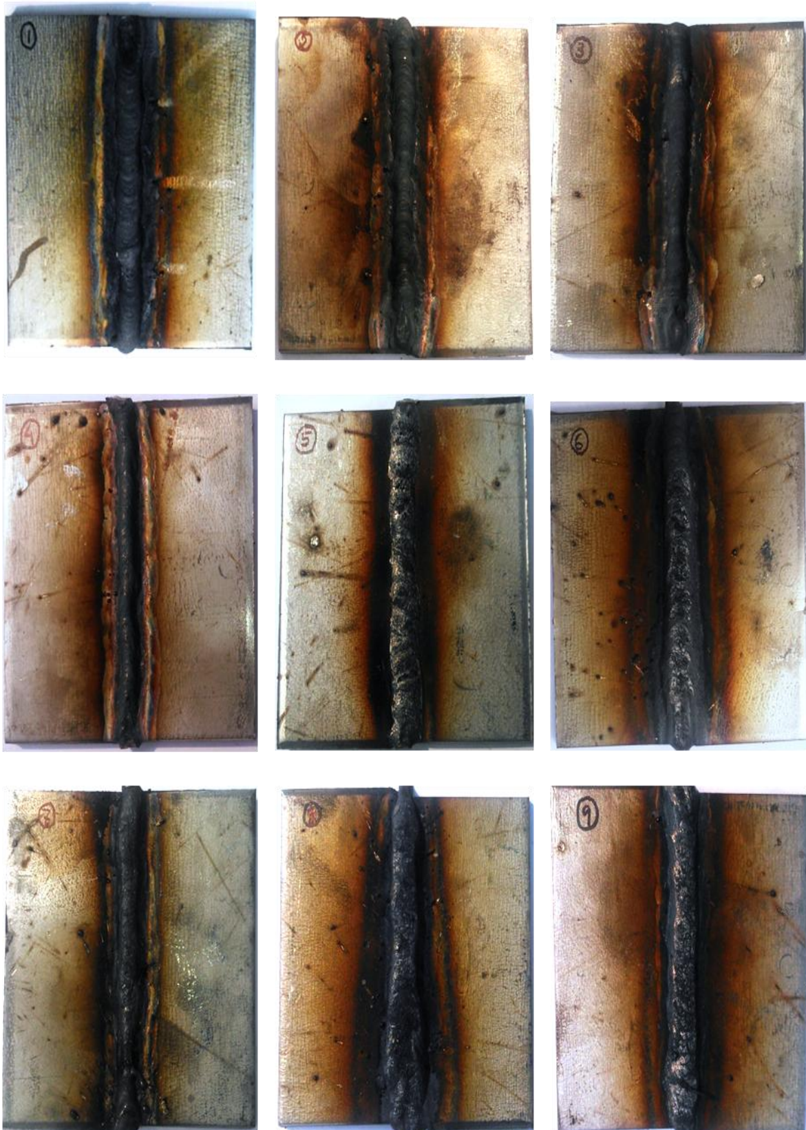
Figure 4.9: Specimens of AISI 304 stainless steel after GMAW
