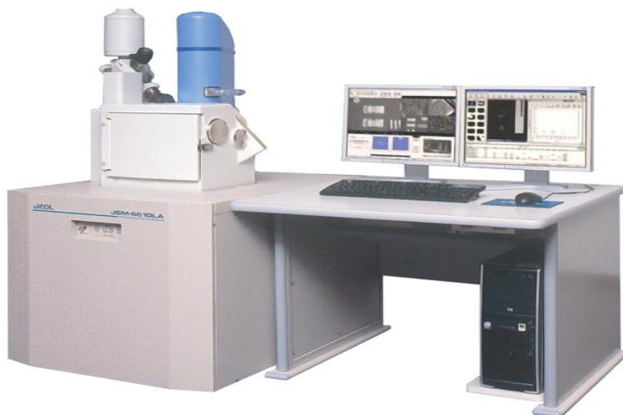
Figure 4.25: Scanning electron microscopy machine (Courtesy: SEM Lab, Indian Institute of Technology, Ropar)
