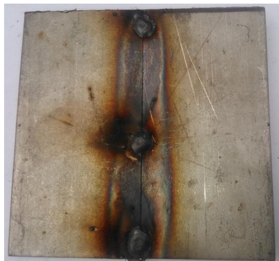
Figure 4.7: Tacking of the welding specimens using GMAW
