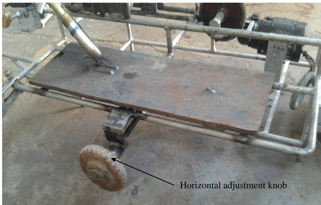
Figure 3.8: Work table for placing the welding specimens
