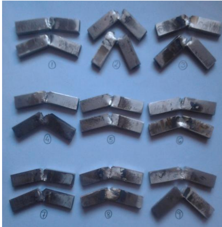
Figure 5.1: Specimens of AISI 304 stainless steel after toughness test
