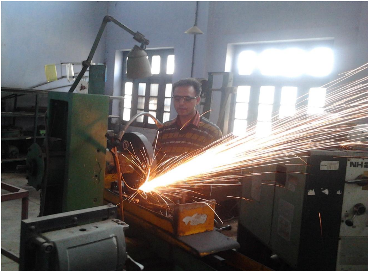
Figure 4.11: Weld bead removal on surface grinder (Courtesy: Central Workshop Thapar University, Patiala)
