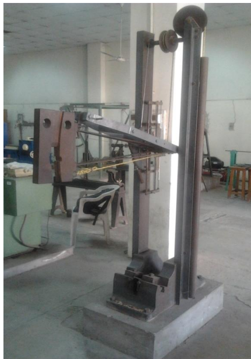
Figure 4.15: Impact testing machine (Courtesy: Solid Mechanics Lab, MED, Thapar University, Patiala)
