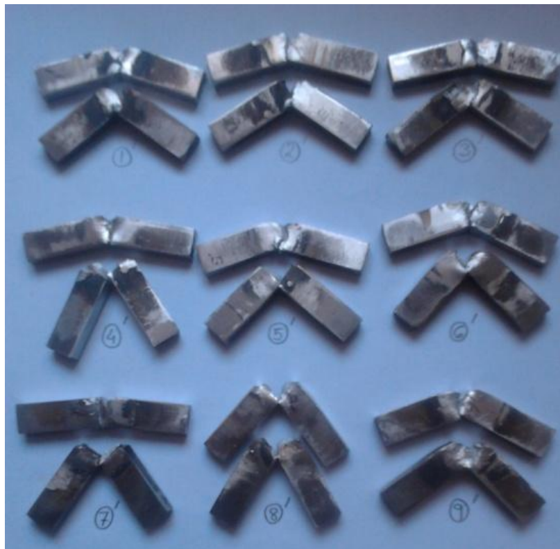
Figure 5.3: Specimens of AISI 316 stainless steel after toughness test
