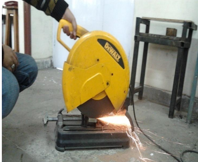
Figure 4.13: Cutting on chop saw (Courtesy: Product Realisation Lab, Indian Institute of Technology, Ropar)
