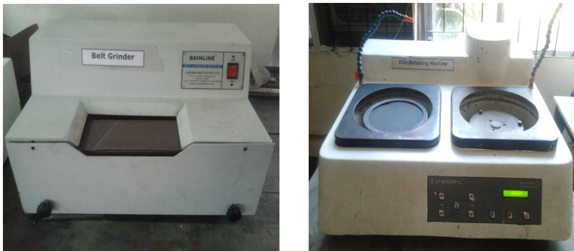
Figure 4.18: Belt grinder and disc polishing machine (Courtesy: Material Science Lab, Indian Institute of Technology, Ropar)
