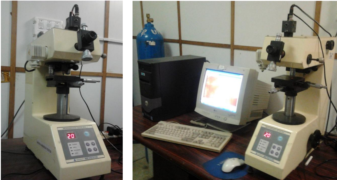
Figure 4.19: Microhardness testing machine (Courtesy: Central Workshop Thapar University, Patiala)
