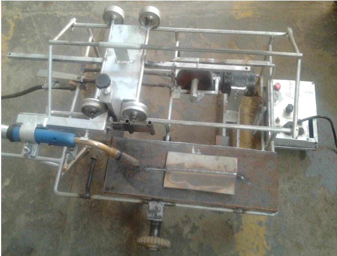
Figure 3.2: Gas metal arc welding fabricated setup
