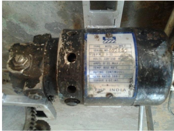
Figure 3.3: Motor used for drive movement in automatic GMAW
