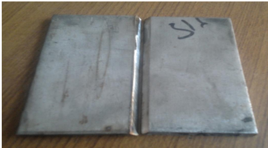
Figure 4.6: Specimens after edge preparation
