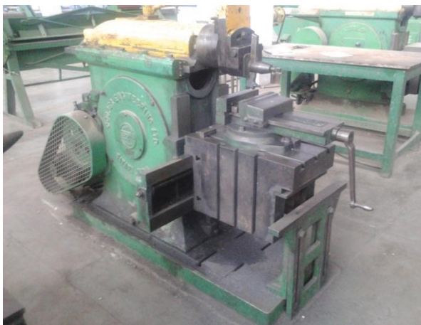
Figure 4.14: Shaper machine used for making v-notch and impact test samples
