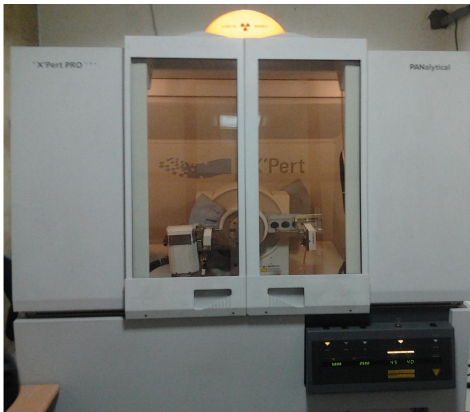
Figure 4.21: X-ray diffraction machine (Courtesy: XRD Lab, Indian Institute of Technology, Ropar)
