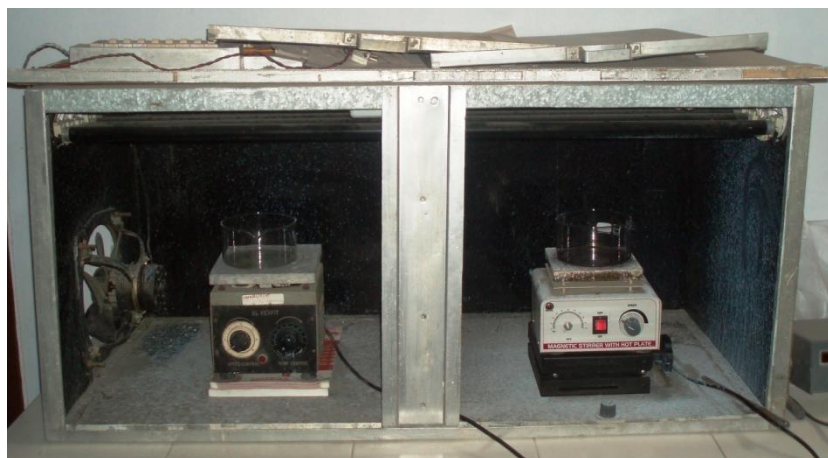
Fig. 2.3. Photograph of the photocatalytic reactor set up
