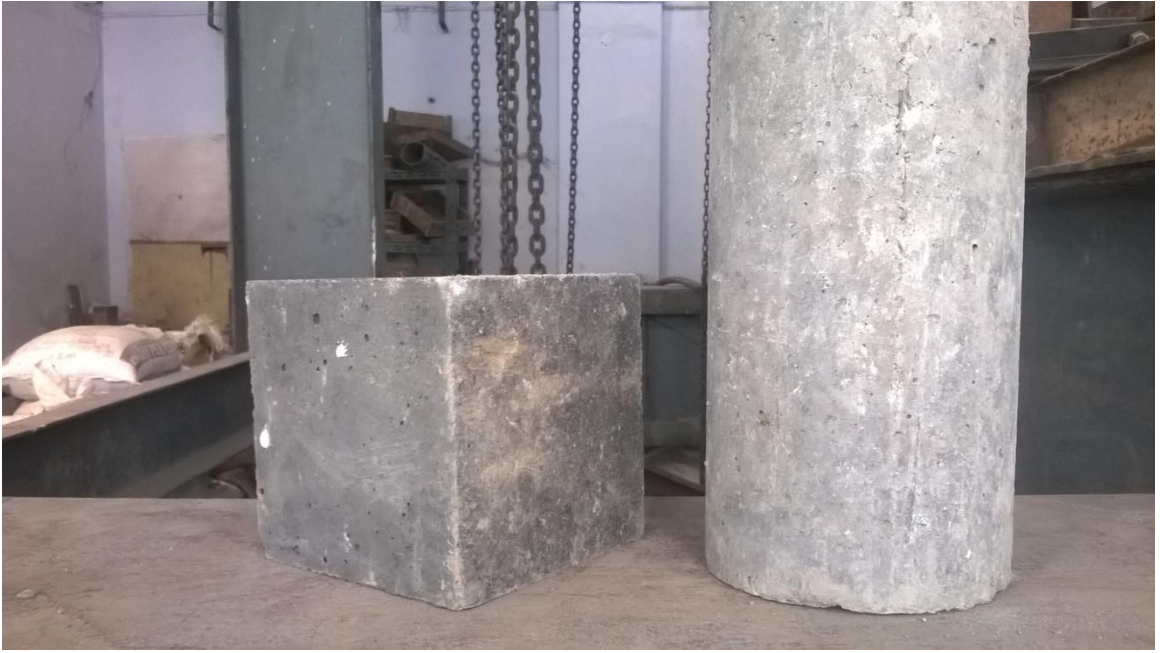
Figure 3.1: Cube 150mm and Cylinder \text{\O}150 \times 300\text{mm}
