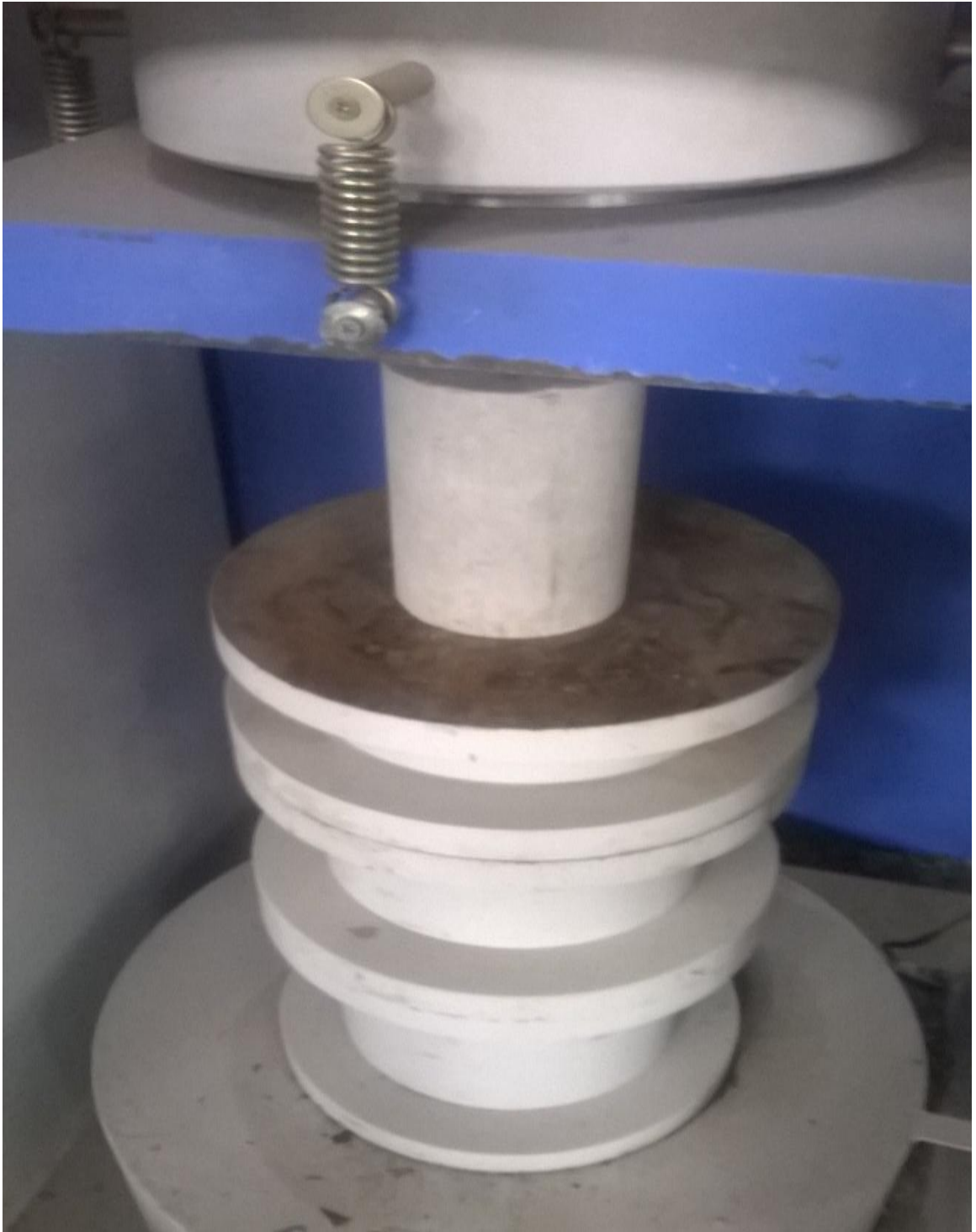
Figure 4.17: Cylinder specimen under compression
