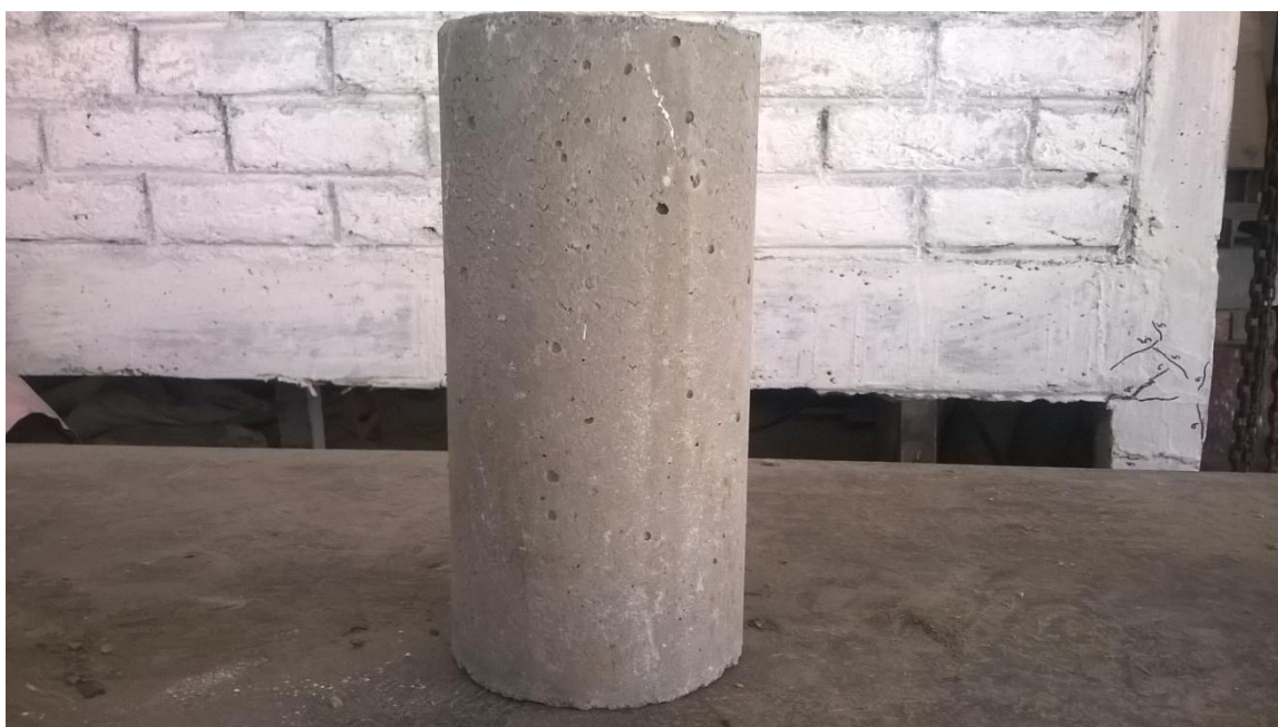
Figure 3.1(b): Ø100x200mm Cylinder
