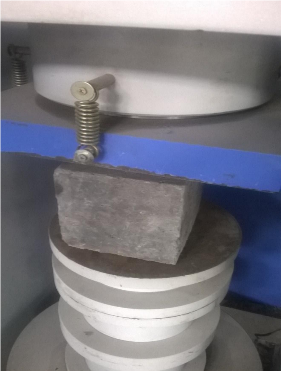
Figure 4.18: Cube Specimen under compression
