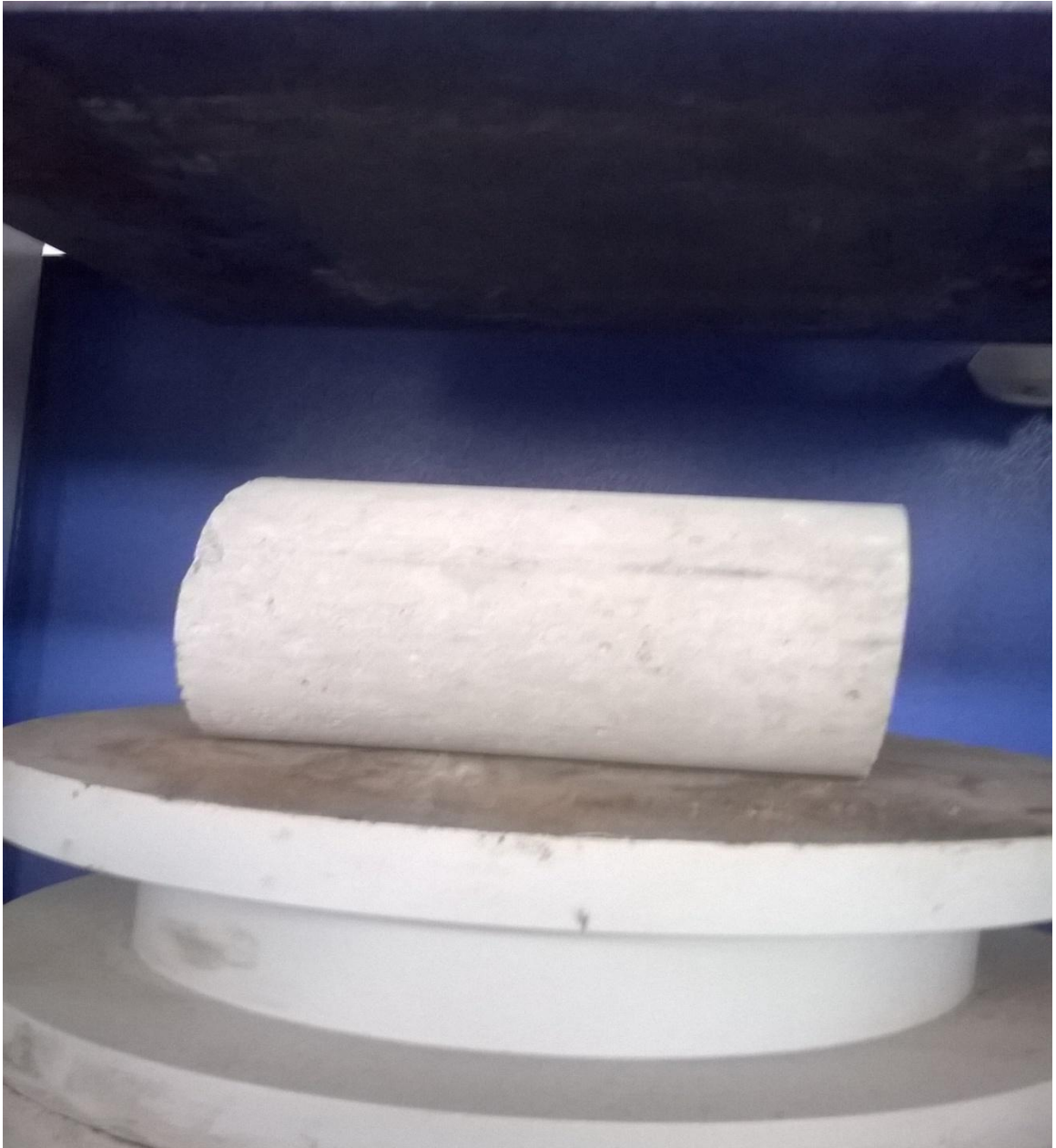
Figure 4.19: Cylinder specimen under splitting tension
