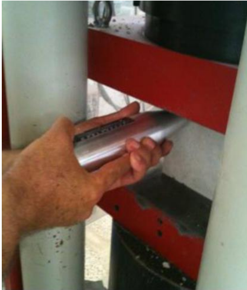
Figure 4.21: Rebound hammer test
