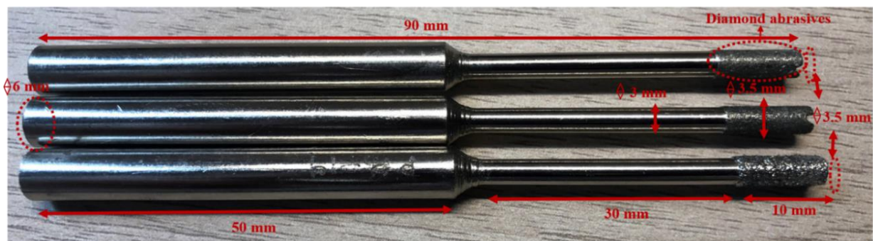
Figure 3.2 three distinct diamond abrasive grit size hollow drill tools
