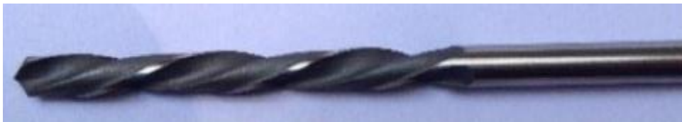
Figure 2.2 Surgical drill bit used for conventional bone drilling [20]
