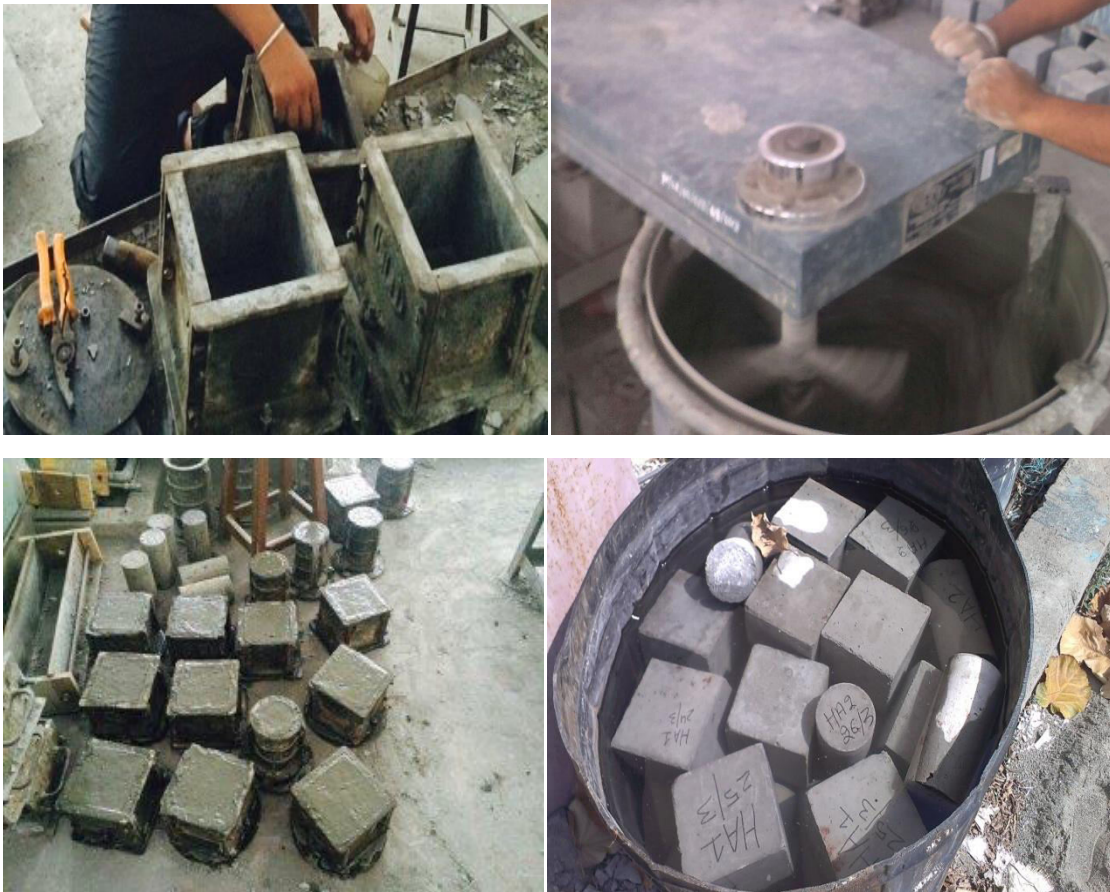
Fig. 3.7: ( A oiling ,B mixing ,C casting ,D curing )
