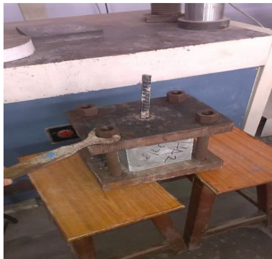
Fig. 3.11: Test Setup for Pull out Strength Test
