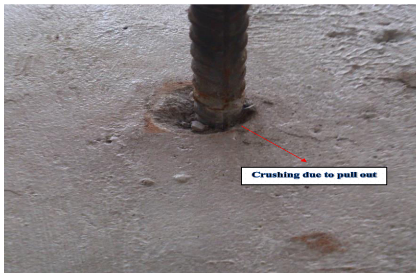
Fig.3.13 (a,b,c): Crushing due To Pull out Bar Lugs after Pull out Test
