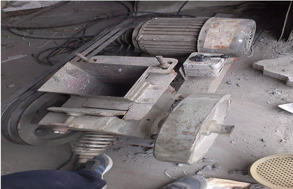
Fig. 3.2: Jaw crusher to obtain RCA
