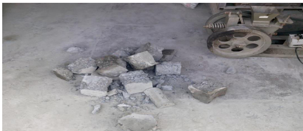
Fig. 3.1: Waste concrete rubble for obtaining RCA
