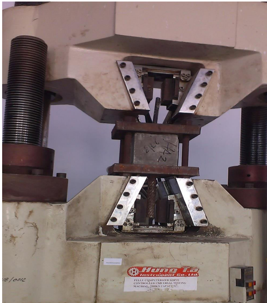
Fig 3.10: Pullout testing machine
